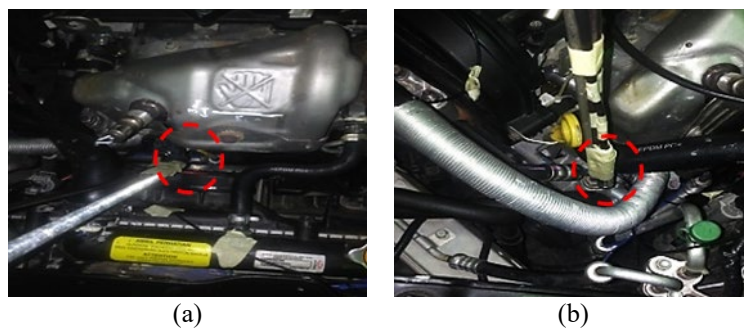
Figure 7: Position of the microphone near the (a) compressor and (b) power steering of the vehicle system.
