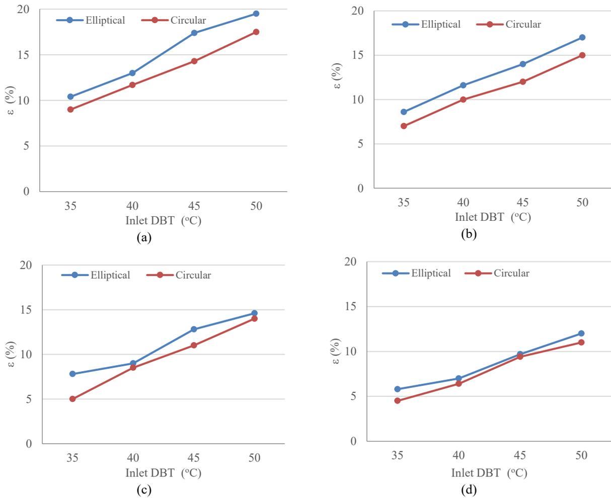
**Figure 11.** Comparison of effectiveness between circular and elliptical OHP heat exchangers for different air velocities (a) 0.5 m/s, (b) 1 m/s, (c) 1.5m/s, and (d) 2 m/s.
