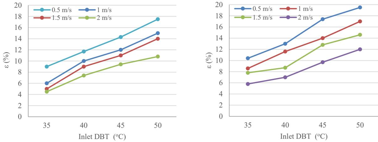
**Figure 10.** Thermal effectiveness vs, inlet DBT for the OHPHX evaporator on sensible using (a) circular tubes, and (b) elliptical tubes.
