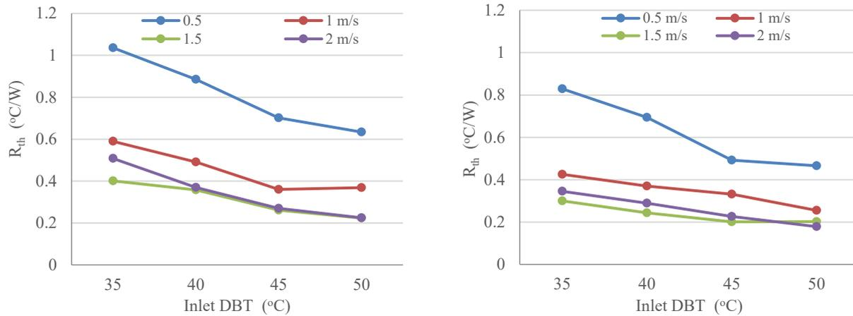
Figure 12. The thermal resistance vs inlet DBT of the OHP evaporator for (a) conventional tube and (b) elliptical tube.
