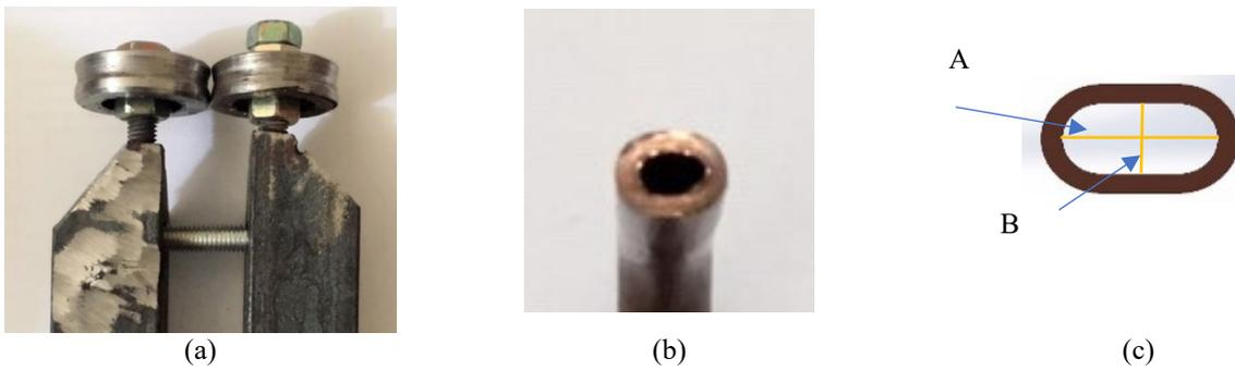
Figure 3. (a) The tool used to form the oval tubes, (b) oval cross-sectional area of copper tube, (c) schematic oval cross-sectional area.
