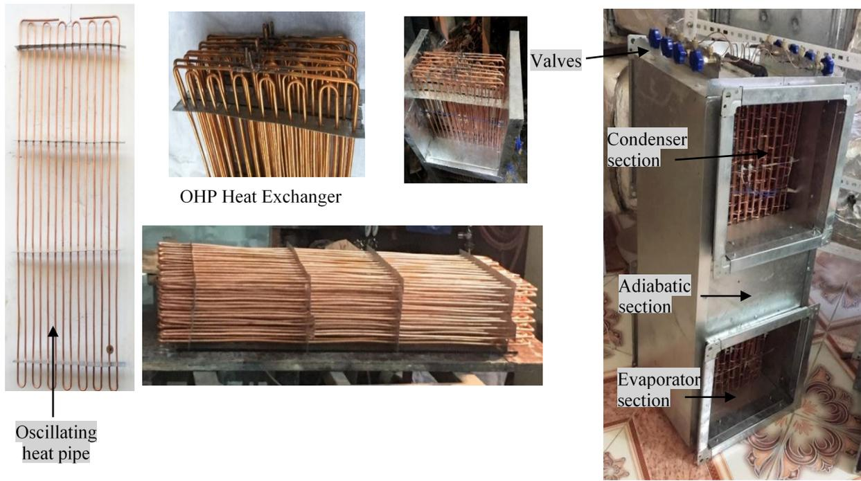
**Figure 5.** Pictures of OHP heat exchanger.
