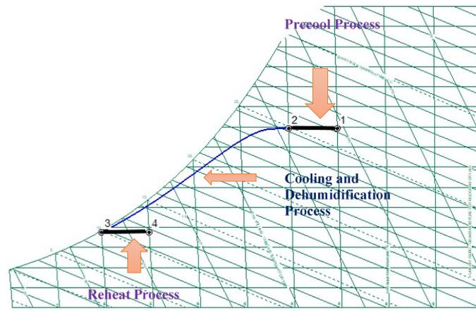
Figure 7. Air thermodynamic processes on psychometric chart.
