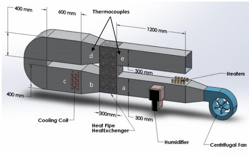
Figure 2. Schematic diagram of HVAC system.
