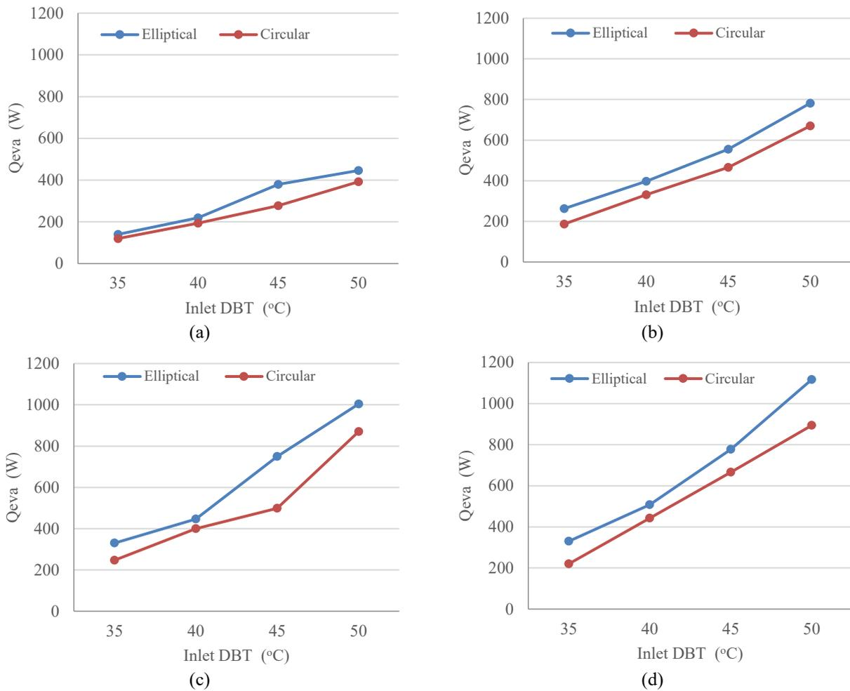
**Figure 14.** The  $Q_{eva}$  vs inlet DBT air velocity for the elliptical and circular OHPHX evaporator at (a) 0.5 m/s, (b) 1 m/s, (c) 1.5 m/s, and (d) 2 m/s.
