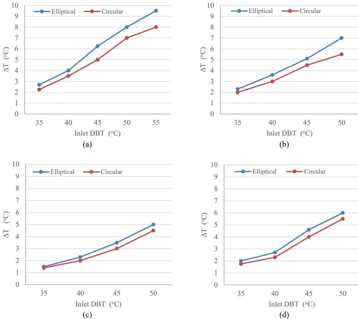
**Figure 9.** The comparison between elliptical and circular OHPHX for temperature difference evaporator section at constant air velocity of (a) 0.5 m/s, (b) 1 m/s, and (c) 1.5 m/s, and (d) 2 m/s.
