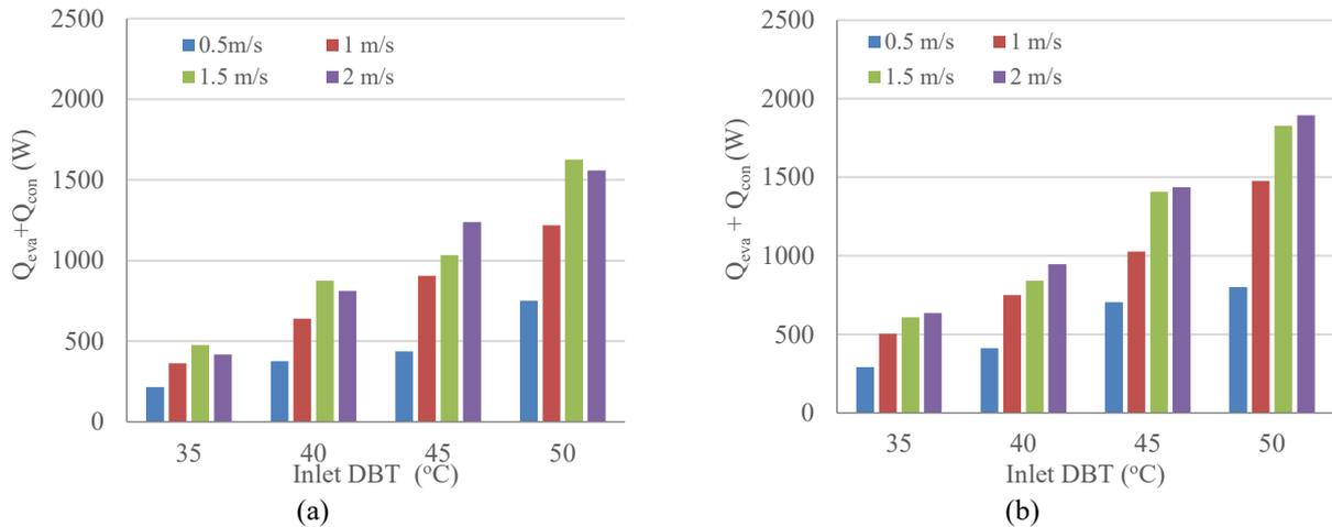
**Figure 15.** Total energy saving vs inlet DBT for the OHPHX evaporator using (a) circular tube with and, (b) elliptical tube.
