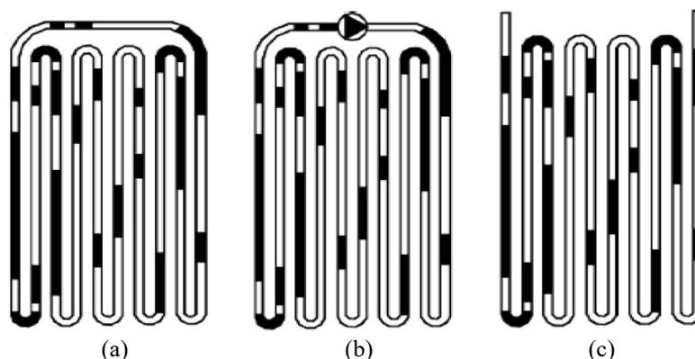
**Figure 1.** Types of OHP; (a) closed-end OHP, (b) OHP with check vale, and (c) open-end OHP.
