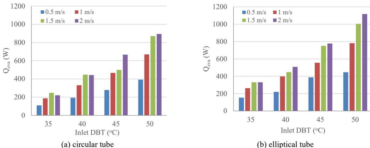
Figure 13.  $Q_{eva}$  vs inlet DBT for evaporator section of the OHPHX.
