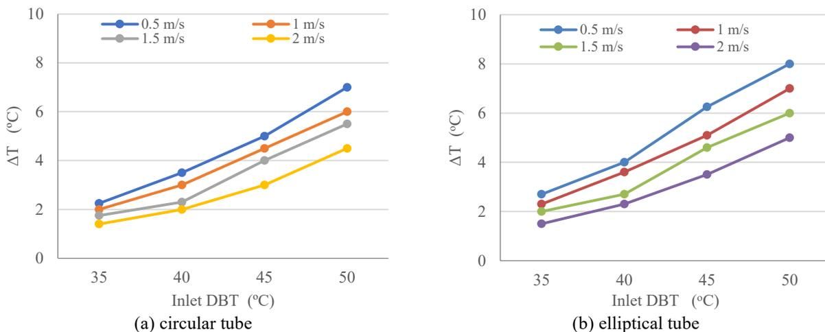
Figure 8. The air temperature difference vs inlet DBT for the OHPHX evaporator for different inlet air velocities.
