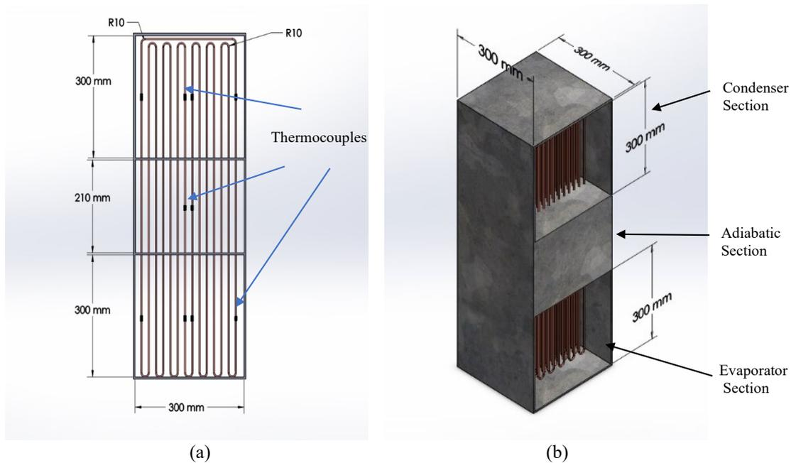
Figure 4. Schematic of (a) oscillating heat pipe and (b) oscillating heat pipe heat.
