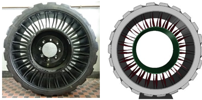
Figure 4. The non-pneumatic (a) tyre and its (b) model (NPT_0).
