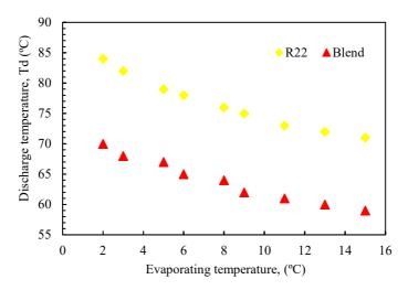
Figure 6. Variation in compressor discharge temperature.
