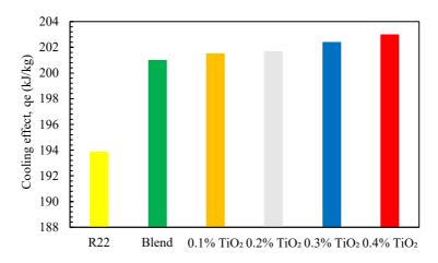
Figure 11. Variation of cooling capacity.
