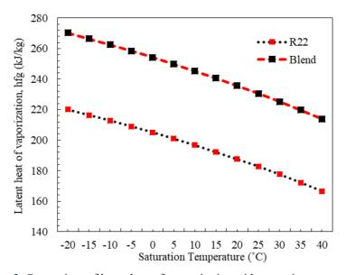
Figure 2. Comparison of latent heat of vapourisation with saturation temperature.
