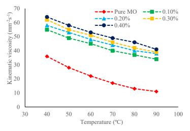
Figure 3. Effect of nanoparticles on the kinematic viscosity of mineral oil with temperature.
