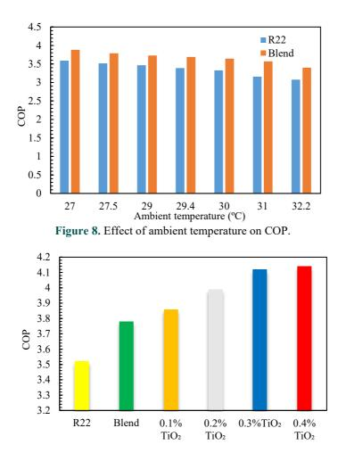
Figure 9. Comparison of COP for selected nanolubricant.
