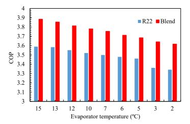
Figure 7. Variation of COP with an evaporator temperature.
