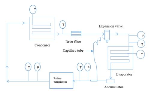
Figure 5. Experimental line diagram.
