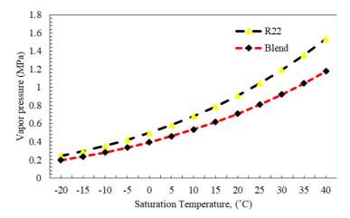
Figure 1. Comparison of vapour pressure with saturation temperature.
