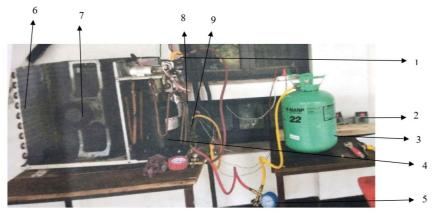
1. kWh meter, 2. Temperature controller, 3. refrigerant cylinder, 4. compressor, 5. pressure gauge, 6. condenser coil, 7. condenser fan, 8. K type thermocouple, 9. expansion valve
