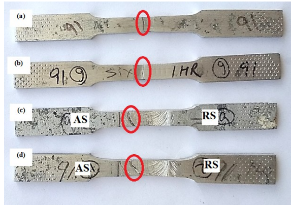
Figure 8. Tensile specimen after testing (a) base metal, (b) base metal heat treated, (c) as-welded joint and (d) PWHT joint.
