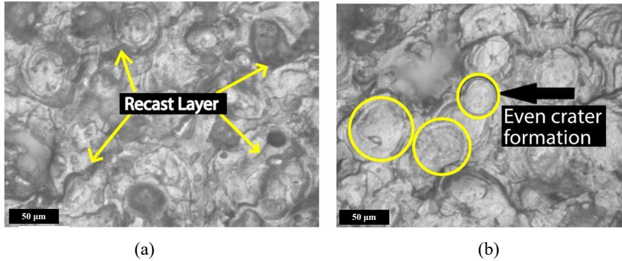
**Figure 9.** Comparison of surface character traits of the machined workpiece using optical microscope (a) without powder, (b) with Al<sub>2</sub>O<sub>3</sub> powder size 10 µm and concentration 6 gm/litre
