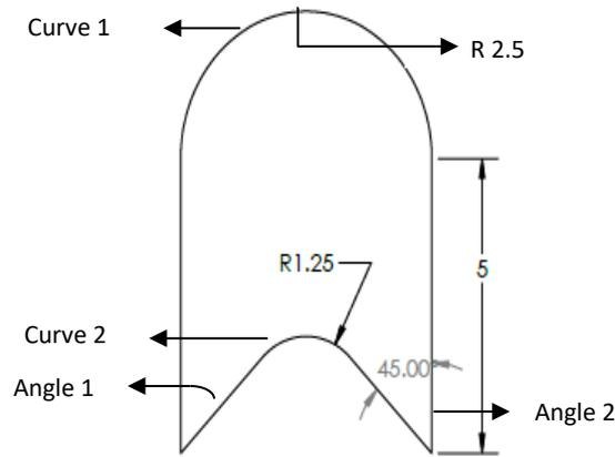
**Figure 1.** CAD geometry of the workpiece profile.
