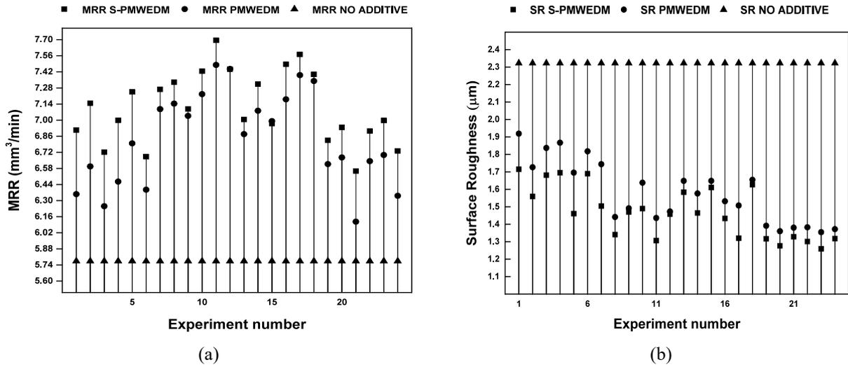
Figure 6. Variation in (a) MRR and (b) SR with the addition of powder and surfactant.
