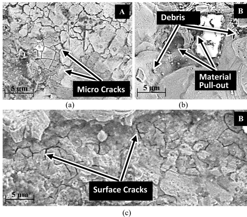
**Figure 11.** SEM images of work piece after machining showing the surface cracks and debris produced after machining (a) without additives and (b), (c) with  $\text{Al}_2\text{O}_3$  (10 micron - 6 g/l).
