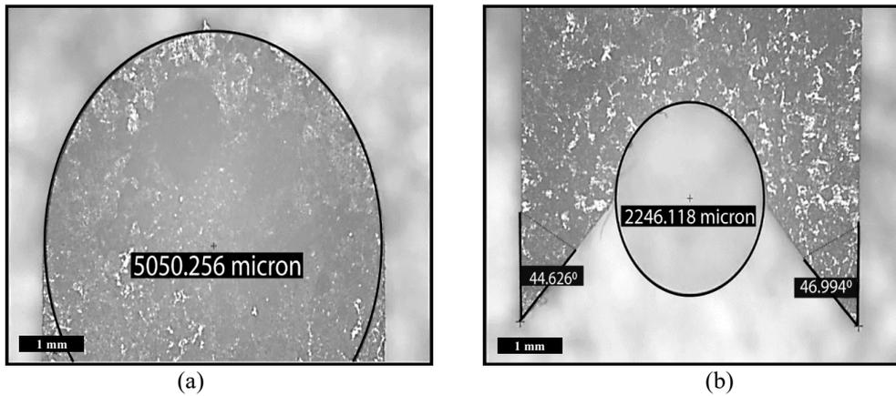
Figure 7. Dimension measurement of (a) external curve (b) internal curve and angles using optical microscope.
