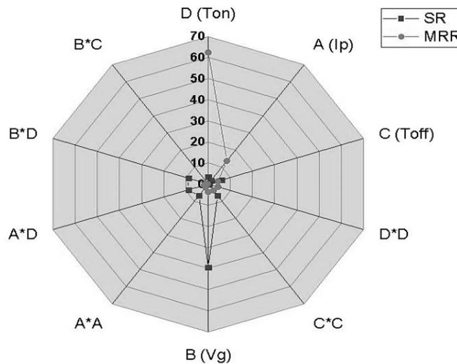
Figure 2. Graph representing the percentage contribution of different electrical parameters on MRR and SR.
