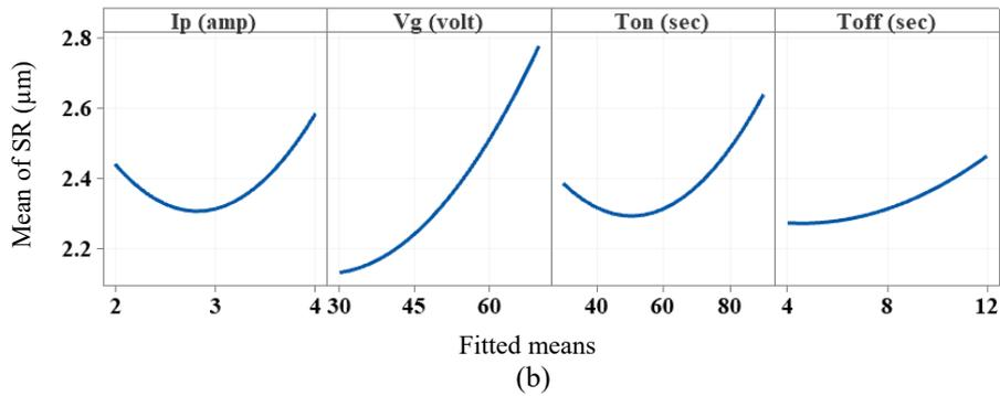
Figure 4. (a) Interaction plot and, (b) main effect plot for SR.
