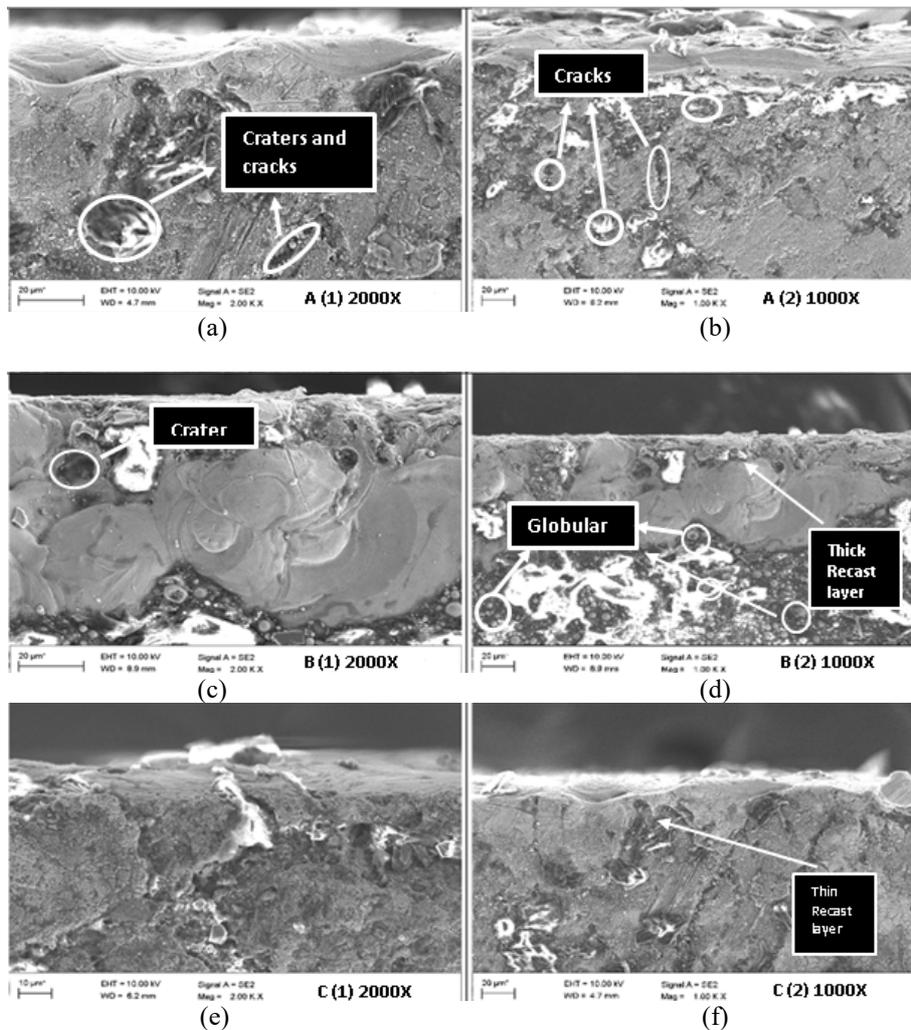
**Figure 10.** SEM images of workpiece after machining (a), (b) without additives (c), (d) with Al<sub>2</sub>O<sub>3</sub> (10 micron- 6 g/l) (e), (f) with surfactant and Al<sub>2</sub>O<sub>3</sub> (10 micron- 6g/l).
