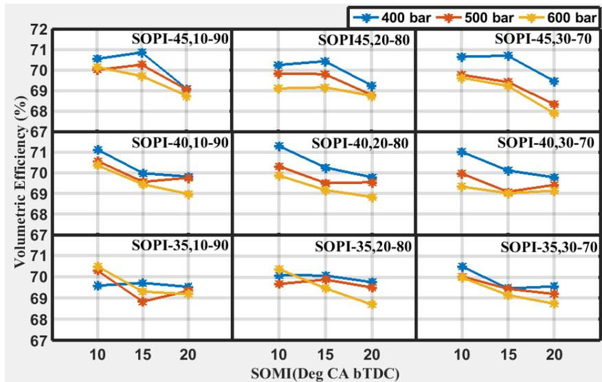
**Figure 7.** Effect of SOPI, SOMI and injection quantity on volumetric efficiency for different IPs.
