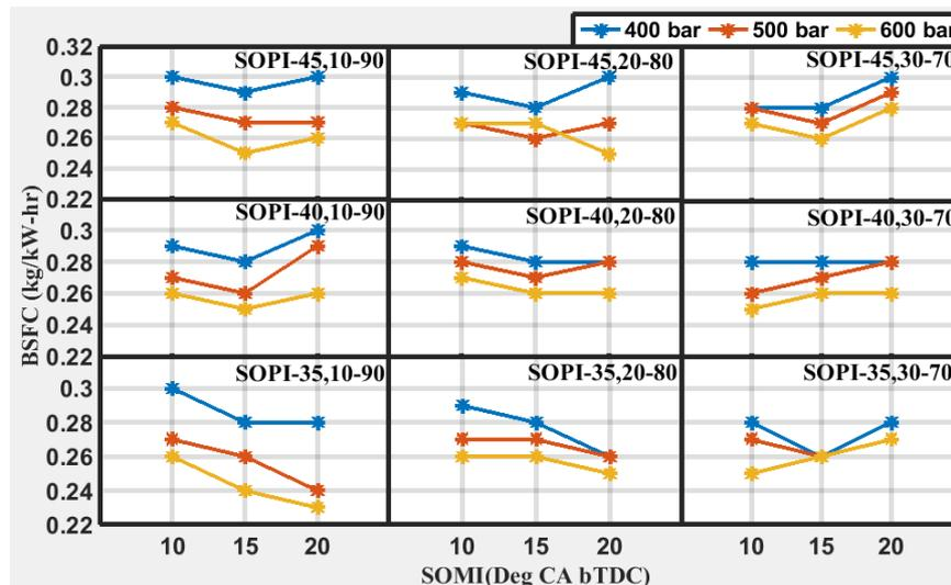
Figure 5. Effect of SOPI, SOMI and injection quantity on BSFC for different IPs.
