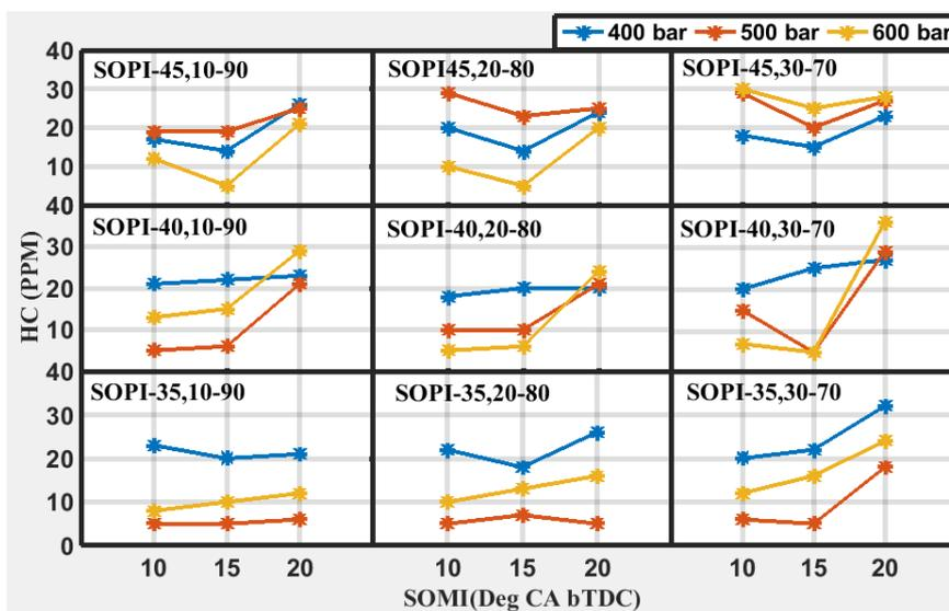
Figure 9. Effect of SOPI, SOMI and injection quantity on HC emission for different IPs.
