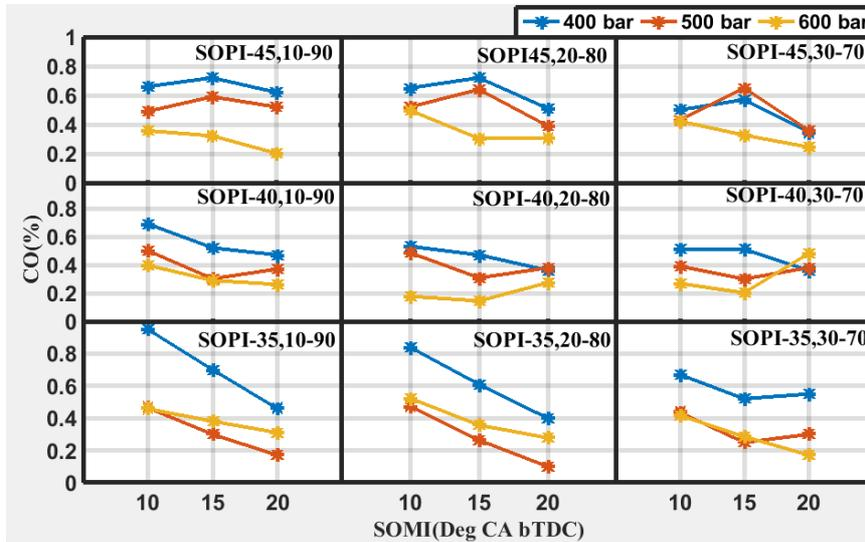
**Figure 10.** Effect of SOPI, SOMI and injection quantity on CO emission for different IPs.
