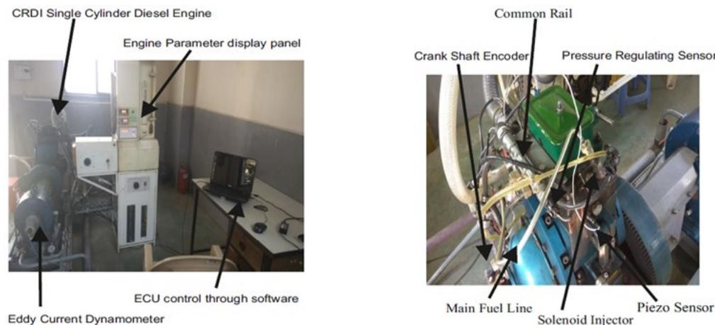
**Figure 1.** Pictorial view of the experimental setup for CRDI single-cylinder diesel engine.
