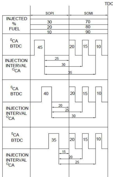
Figure 2. SOMI and SOPI timing and a quantity of injection with injection interval.
