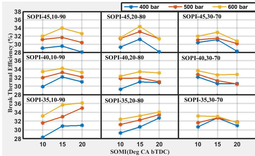
Figure 4: Effect of SOPI, SOMI and injection quantity on BTE for different IPs.
