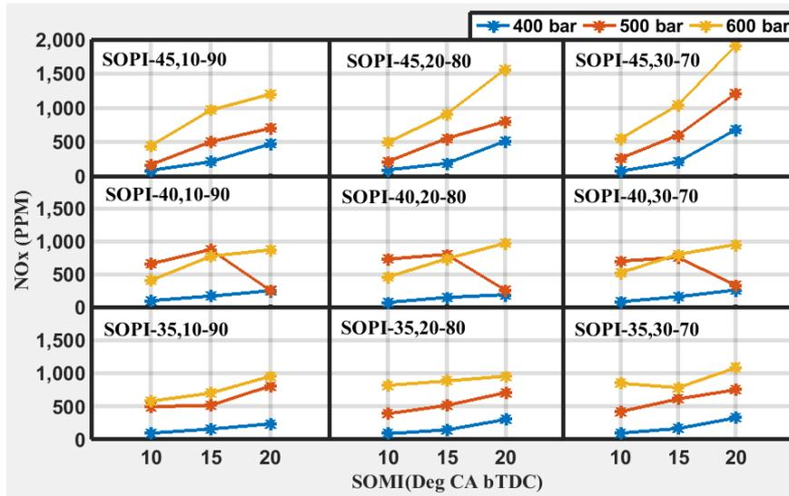
Figure 8. Effect of SOPI, SOMI and injection quantity on NOx emission for different IPs.
