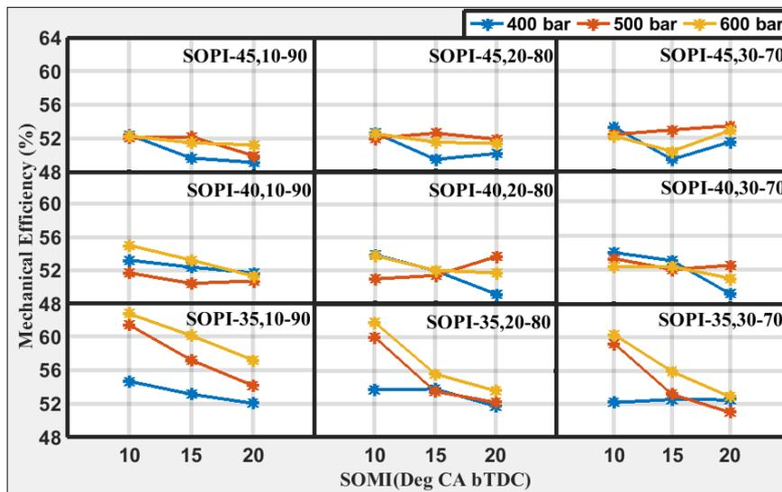
**Figure 6.** Effect of SOPI, SOMI and injection quantity on mechanical efficiency for different IPs.
