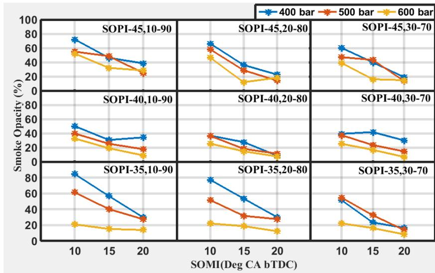
**Figure 11.** Effect of SOPI, SOMI and injection quantity on smoke opacity for different IPs.
