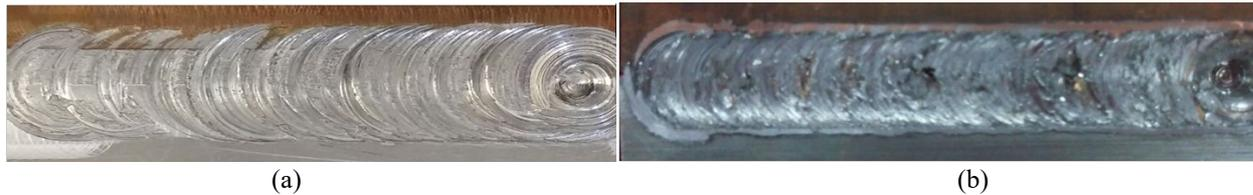
**Figure 8.** Surface morphology of AL-Cu joint fabricated at 1000 rpm under EWW-WPO (with GNPs) at (a) 1000 rpm and, (b) 800 rpm.
