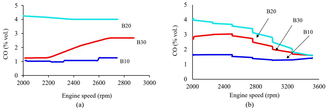
**Figure 9.** CO emission for all tested fuels using (a) sweep test and (b) step test.
