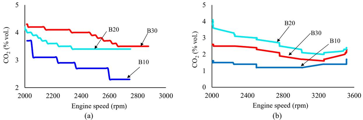
**Figure 8.** CO<sub>2</sub> emission for all tested fuels using (a) sweep test and (b) step test.
