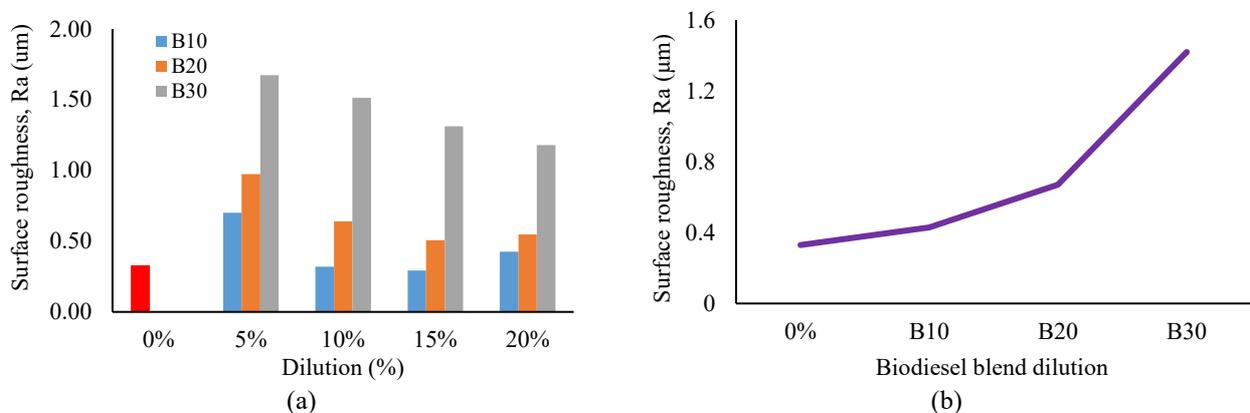
**Figure 5.** Roughness of Ra comparator showing an average profile for various dilutions.
