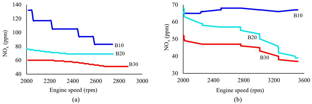
**Figure 10.** NO<sub>x</sub> emission for all tested fuels using (a) sweep test and (b) step test.
