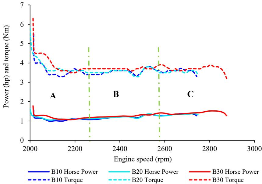
**Figure 6.** Variation in power and torque with engine speed during sweep test.
