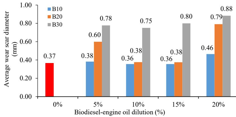
**Figure 3.** Wear Scar Diameter (WSD) for various 20W50 engine oil dilution.
