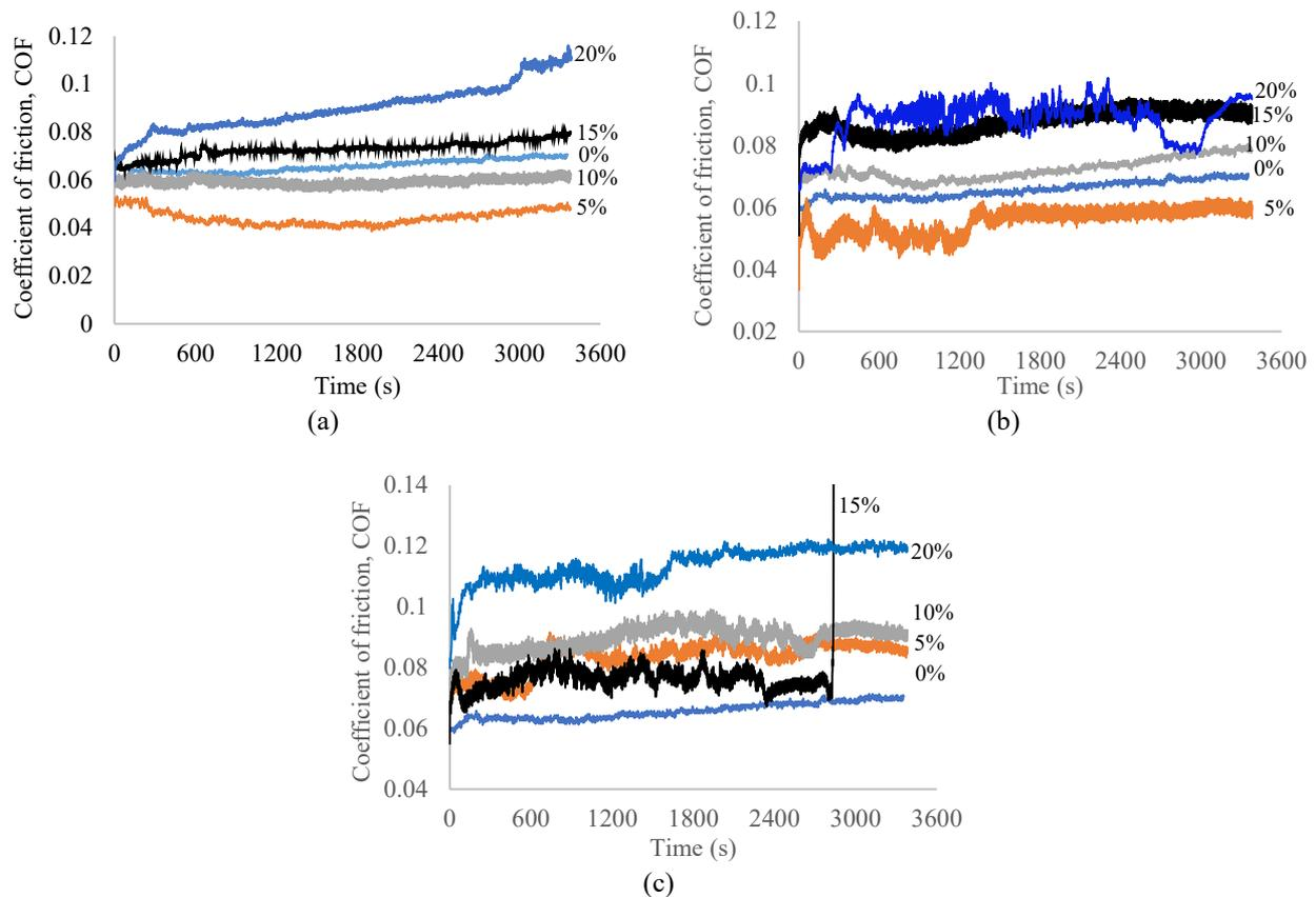
**Figure 2.** Coefficient of friction variation for (a) B10 diluted 20W50 engine oil (b) B20 diluted 20W50 engine oil, and (c) B30 diluted 20W50 engine oil.
