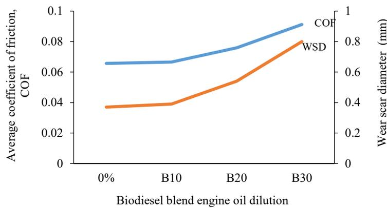
**Figure 4.** Coefficient of friction and wear scar diameter vs biodiesel blend ratio.
