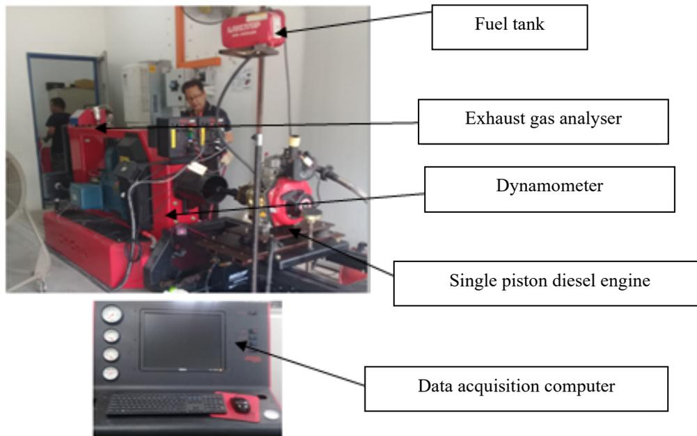
**Figure 1.** Engine dyno set-up.
