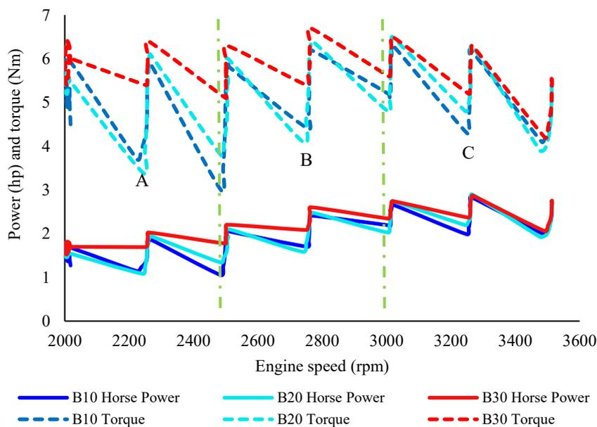
**Figure 7.** Variation in power and torque with engine speed during step test.
