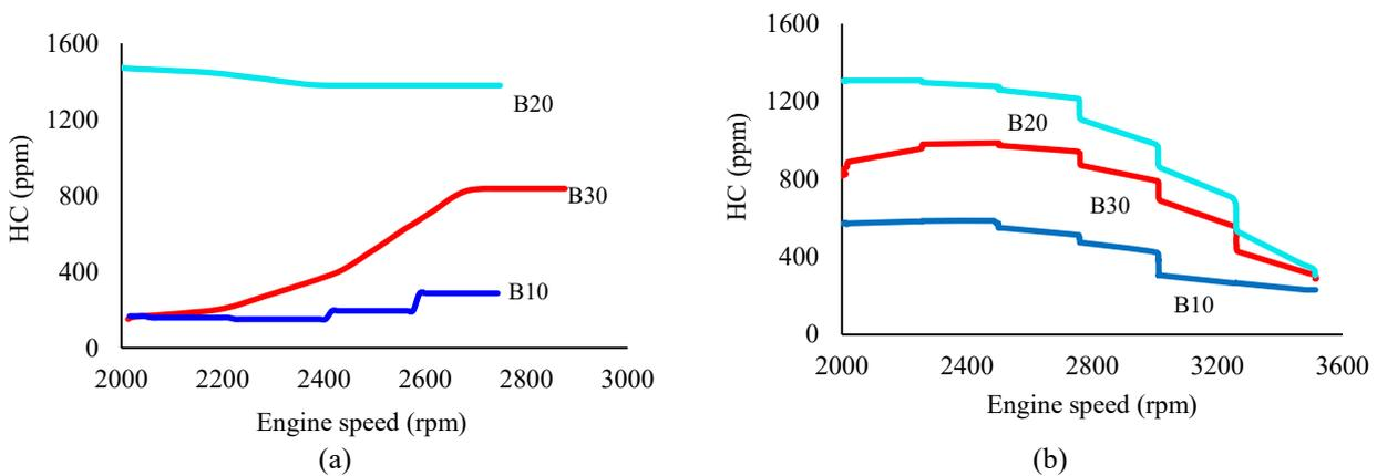
**Figure 11.** HC emission for all tested fuels using (a) sweep test and (b) step test.
