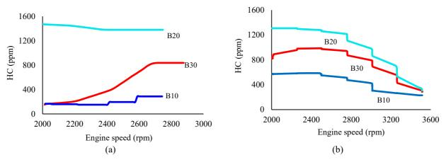
Figure 11. HC emission for all tested fuels using (a) sweep test and (b) step test.
