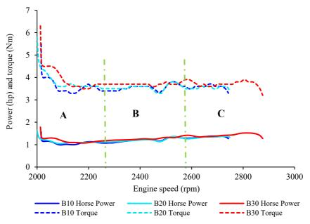
Figure 6. Variation in power and torque with engine speed during sweep test.
