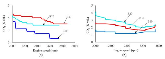
Figure 8. CO<sub>2</sub> emission for all tested fuels using (a) sweep test and (b) step test.
