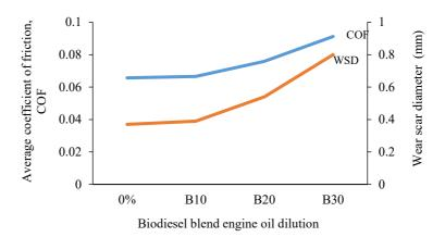
Figure 4. Coefficient of friction and wear scar diameter vs biodiesel blend ratio.
