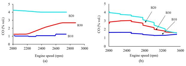
Figure 9. CO emission for all tested fuels using (a) sweep test and (b) step test.
