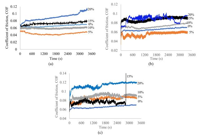
Figure 2. Coefficient of friction variation for (a) B10 diluted 20W50 engine oil (b) B20 diluted 20W50 engine oil, and (c) B30 diluted 20W50 engine oil.
