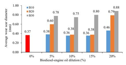
Figure 3. Wear Scar Diameter (WSD) for various 20W50 engine oil dilution.
