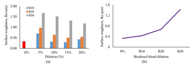
Figure 5. Roughness of Ra comparator showing an average profile for various dilutions.
