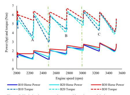
Figure 7. Variation in power and torque with engine speed during step test.
