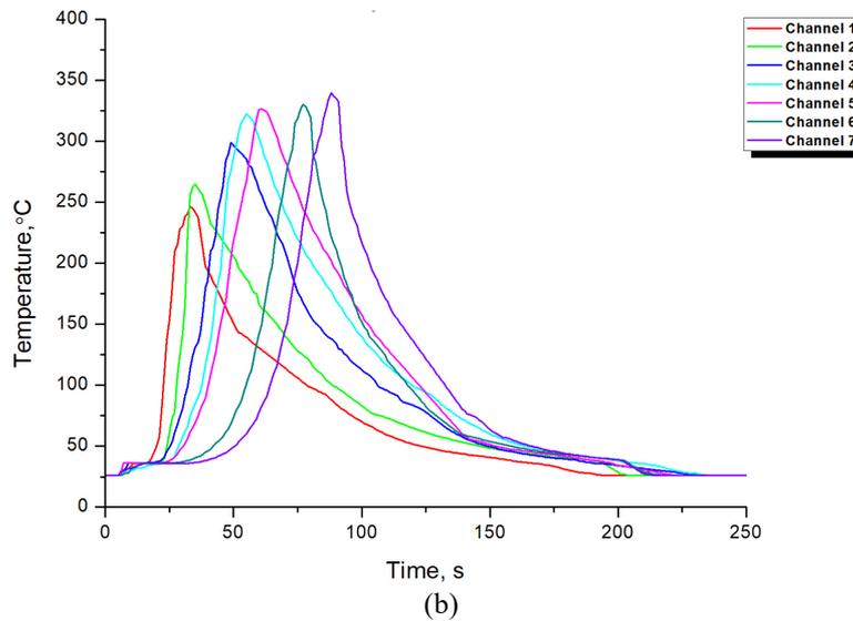
**Figure 4.** Temperature measurement on the (a) advancing side and (b) retreating side for weld process under spindle speed of 750 rpm and welding speed of 130 mm/min.
