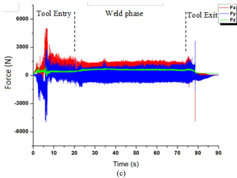
**Figure 3.** Force measurement of all welds processed at spindle speeds of (a) 750 rpm, (b) 850 rpm and (c) 950 rpm at a fixed welding speed of 130 mm/min.
