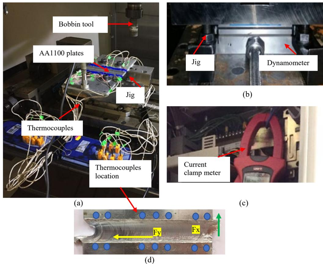
**Figure 1.** (a) Experimental setup with the placement of (b) dynamometer and (c) current clamp meter. (d) Welding force direction ( $F_x$ ,  $F_y$ ).
