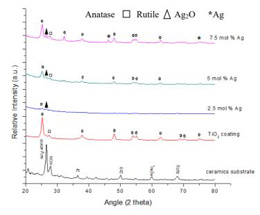
Figure 1: XRD pattern of Ag-TiO2 coated on unglazed ceramic tile substrates.
