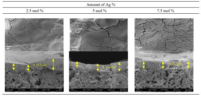
Table 2: SEM/EDX spectra of Ag-TiO2 coating deposited on unglazed ceramics tiles.
