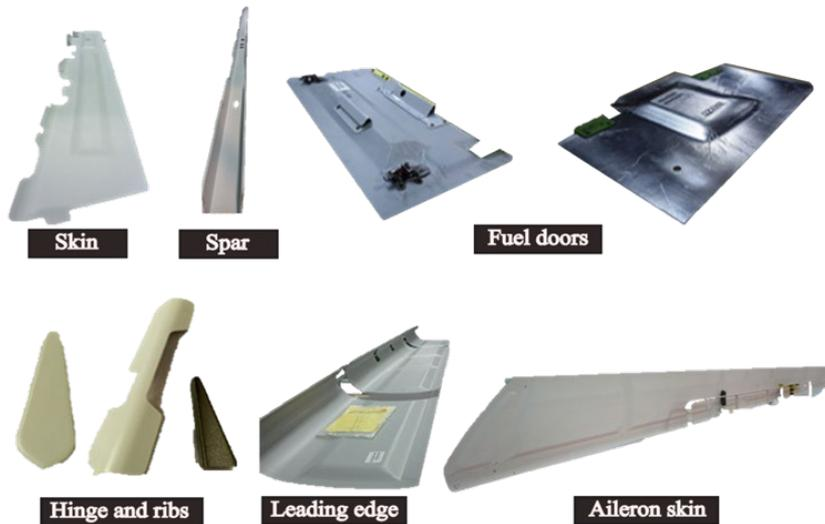
**Figure 3.** Types of aircraft panels in waterjet unit.
