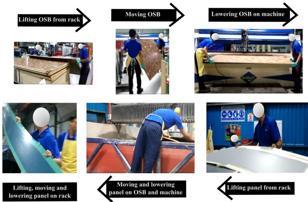
Figure 4. Operation flow in waterjet unit.
