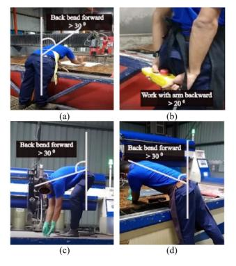
Figure 6. Awkward postures among operators in waterjet unit: (a), (c), (d) back bend forward, (b) work with arm backward.
