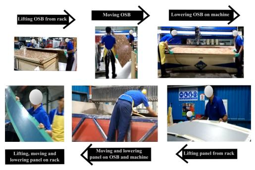
Figure 4. Operation flow in waterjet unit.
