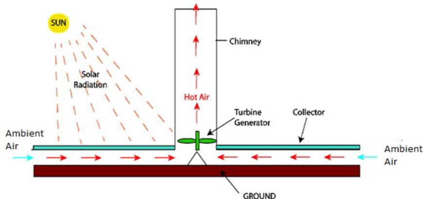
Figure 1. Solar updraft tower concept.
