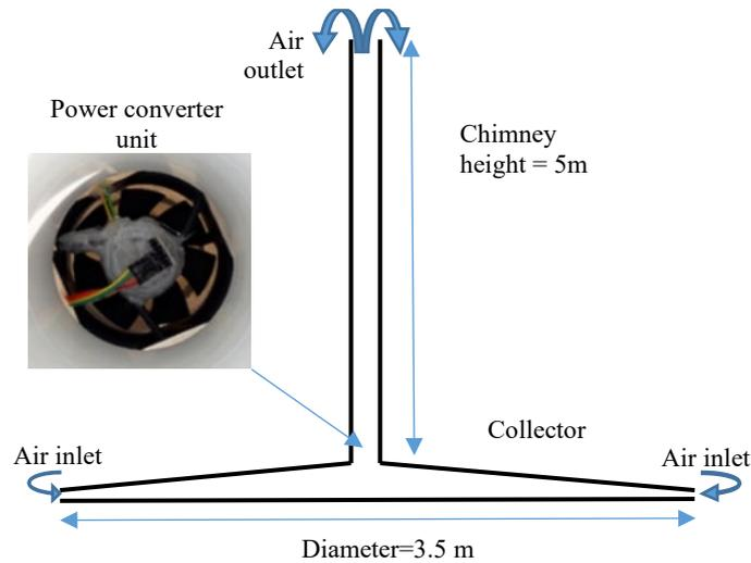
**Figure 5.** Schematic of solar chimney set up.
