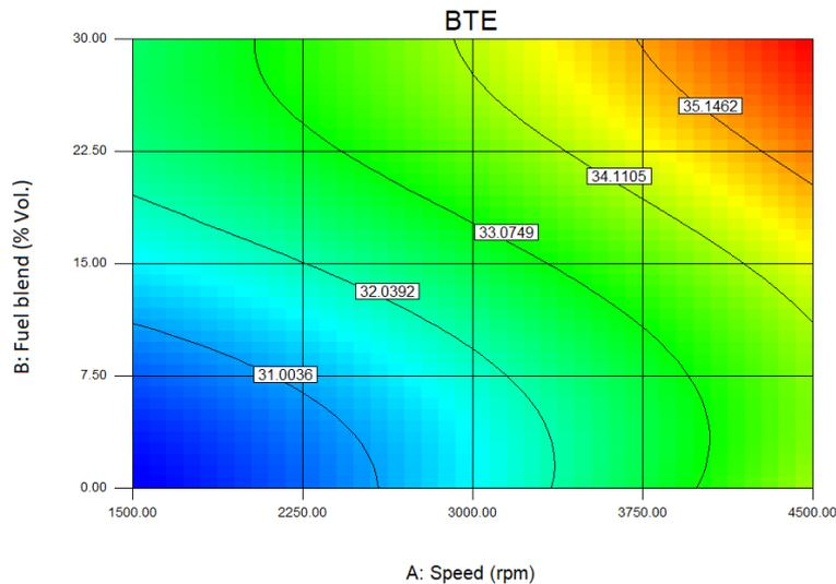
Figure 10. Counter surface plot of brake thermal efficiency against engine speed and fuel blend ratio.
