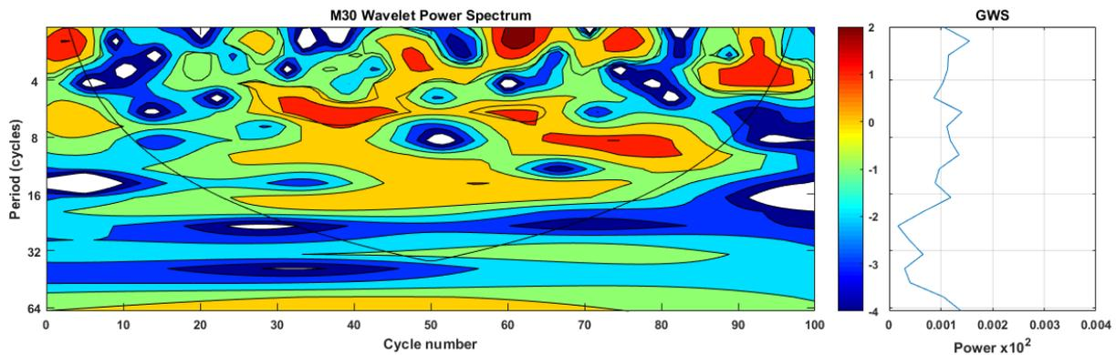
**Figure 14.** Wavelet analysis of IMEP with blended fuel M30 at 2500 rpm engine speed.
