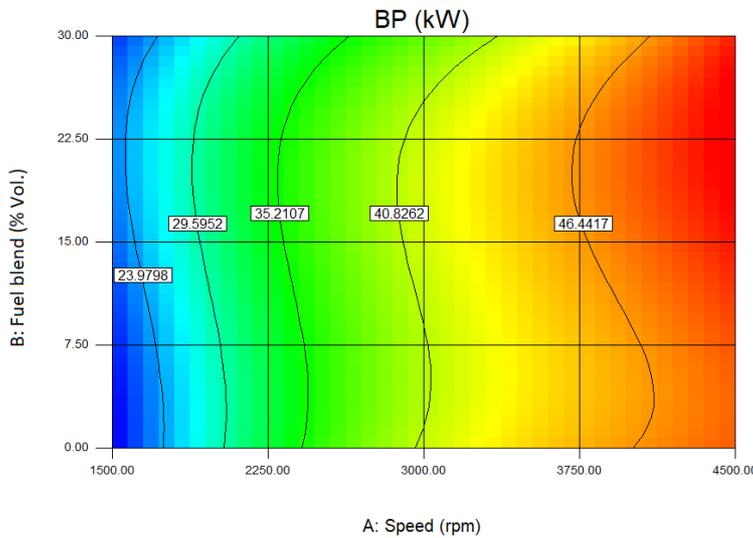
**Figure 4.** Counter surface plot of brake power against engine speed and fuel blend ratio.
