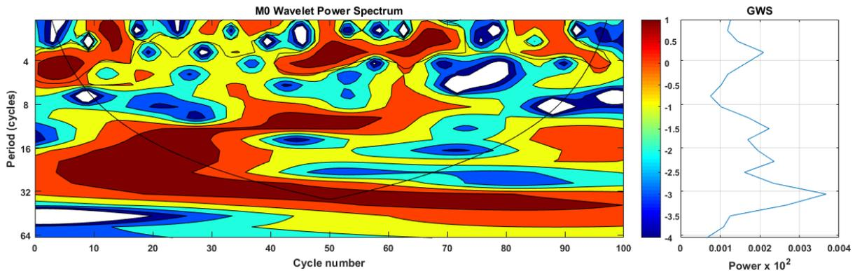
**Figure 11.** Wavelet analysis of IMEP with pure gasoline at 2500 rpm engine speed.
