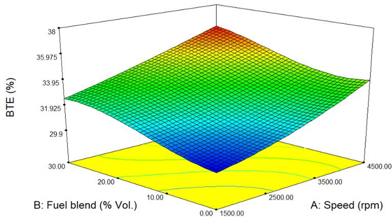
Figure 9. 3D surface plot of brake thermal efficiency against engine speed and fuel blend ratio.
