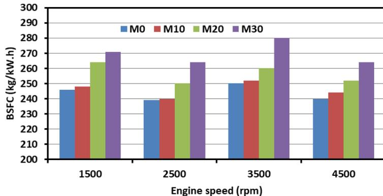
**Figure 5.** Effect of blend ratio on engine BSFC.
