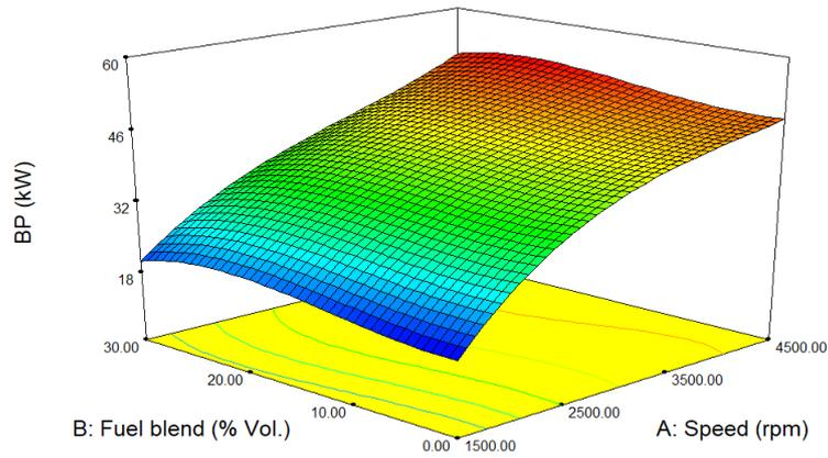
**Figure 3.** 3D surface plot of brake power against engine speed and fuel blend ratio.
