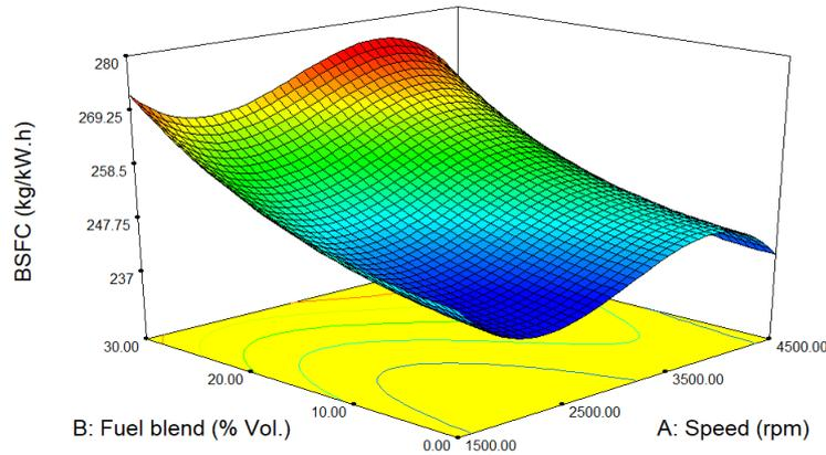
**Figure 6.** 3D surface plot of BSFC against engine speed and fuel blend ratio.
