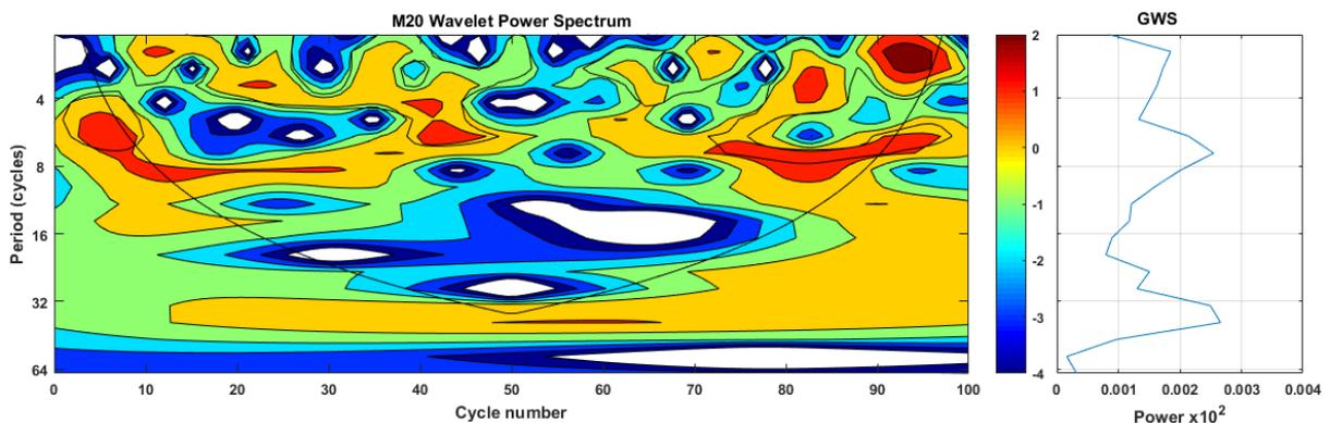
**Figure 13.** Wavelet analysis of IMEP with blended fuel M20 at 2500 rpm engine speed.
