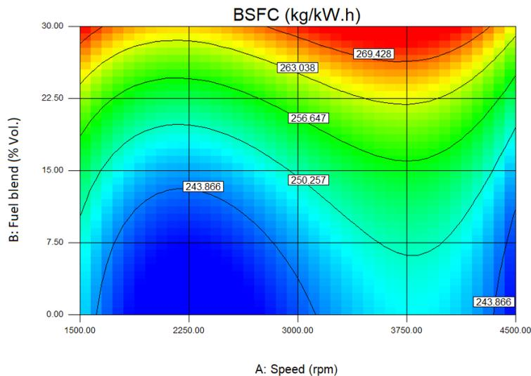
**Figure 7.** Counter surface plot of BSFC against engine speed and fuel blend ratio.
