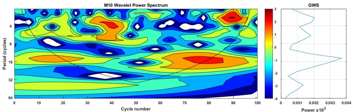
**Figure 12.** Wavelet analysis of IMEP with blended fuel M10 at 2500 rpm engine speed.
