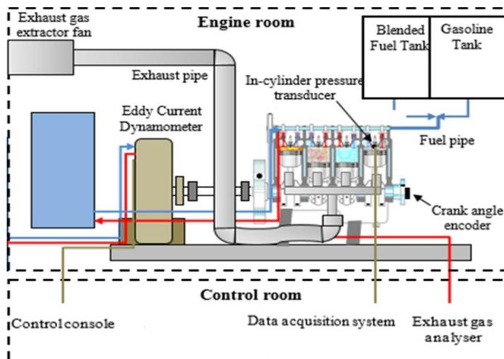
**Figure 1.** Gasoline engine test rig.
