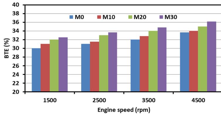
Figure 8. Effect of blend ratio on engine brake thermal efficiency.
