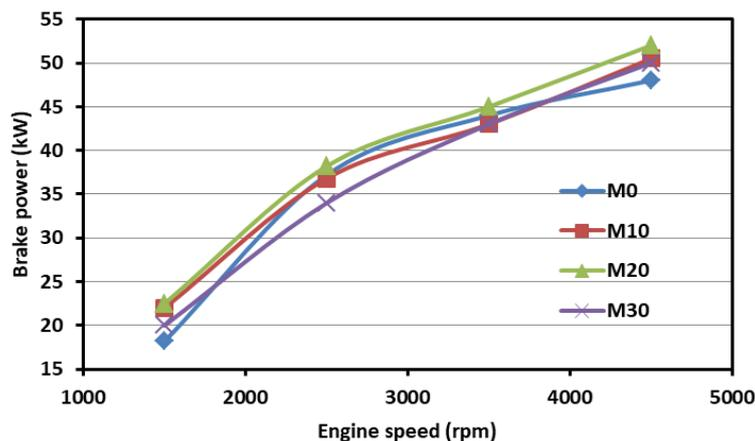
**Figure 2.** Effect of blend ratio on engine brake power.
