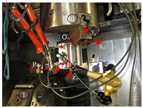
(b) along Y axis of the subsystem 0 from  $P_x$
