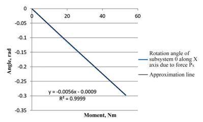
(a) the average angle of rotation along the X-axis of subsystem 0 from  $P_x$
