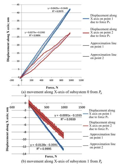
Figure 3. Fragments of experiment results to determine e coordinate matrix and the angular matrix  $\xi$  of compliance of subsystem 0 and 1.
