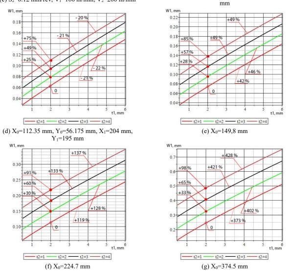
Figure 5. The influence of technological and design factors on the value of distortion of the performed diametric size in two-carriage adjustment.
