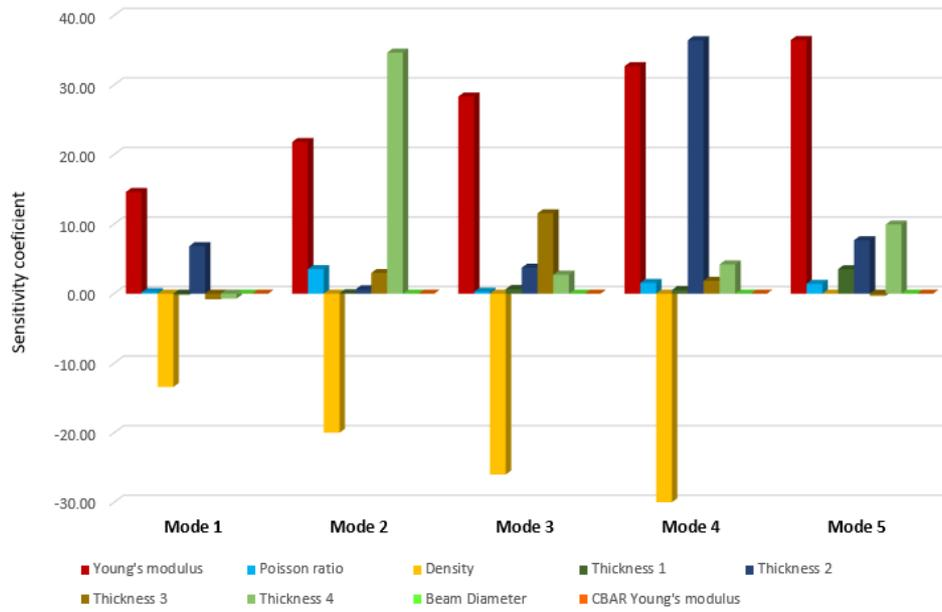
Figure 12. Sensitivity coefficients for potential updating parameters of BIW model with CBAR elements.
