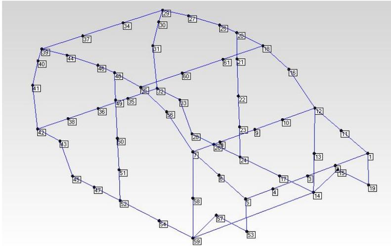
**Figure 3.** An experimental model of BIW structure.
