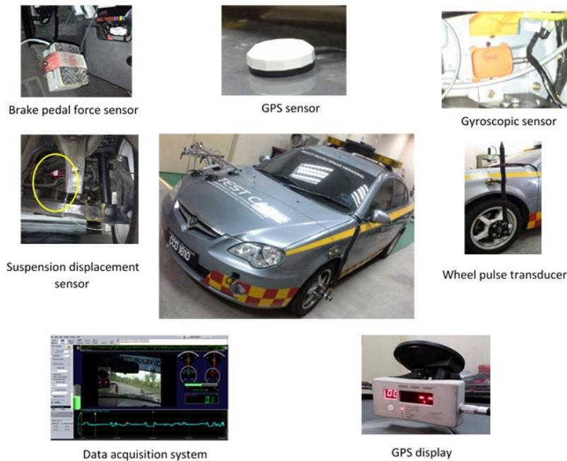
**Figure 4.** Experimental vehicle and instrumentations.
