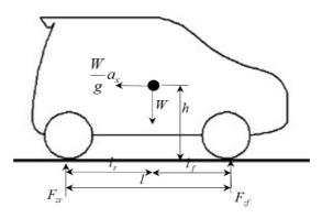
Figure 2. Free body diagram of the car on the level ground
