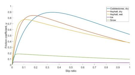
Figure 1. Slip-friction curve for different road surfaces at a linear speed of 10 m/s [12].
