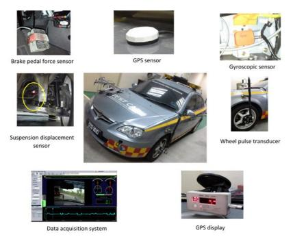
Figure 4. Experimental vehicle and instrumentations.
