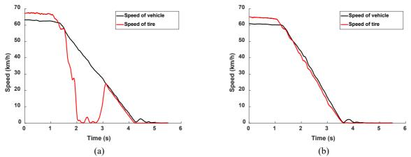
Figure 9. Speed of the car and wheel during emergency braking for (a) wet surface and (b) dry surface condition.
