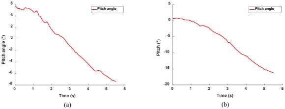
Figure 10. Pitch angle of the vehicle during emergency braking for (a) wet surface and (b) dry surface condition.
