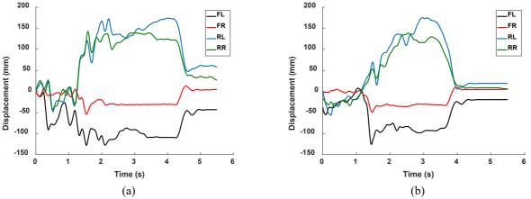
Figure 11. Displacement of each suspension during emergency braking for (a) wet surface and (b) dry surface condition.
