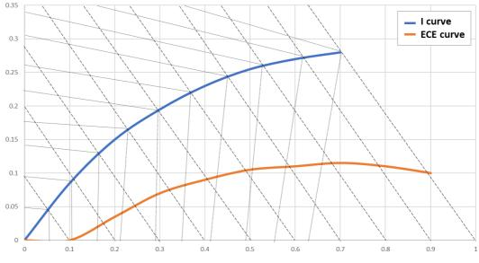
Figure 3. Ideal braking force distribution.
