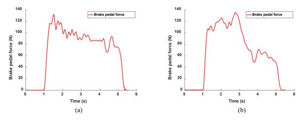
Figure 7. Braking pedal force during emergency braking for (a) wet surface and (b) dry surface condition.
