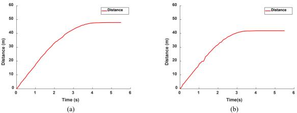
Figure 8. Travelling distance by the car for (a) wet surface and (b) dry surface condition.
