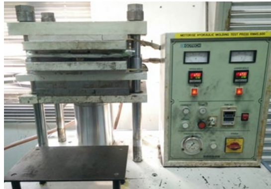
Figure 2. Hotpress machine used in preparing the composite and hybrid composite panel.
