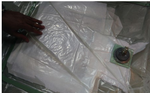
Figure 3. Composite prepreg underwent 1 bar equivalent pressure under vacuum.
