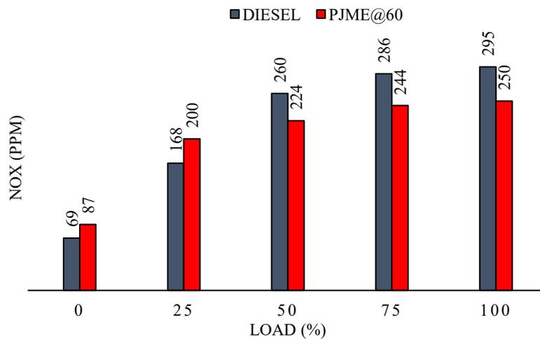
Figure 12. NO vs engine load.
