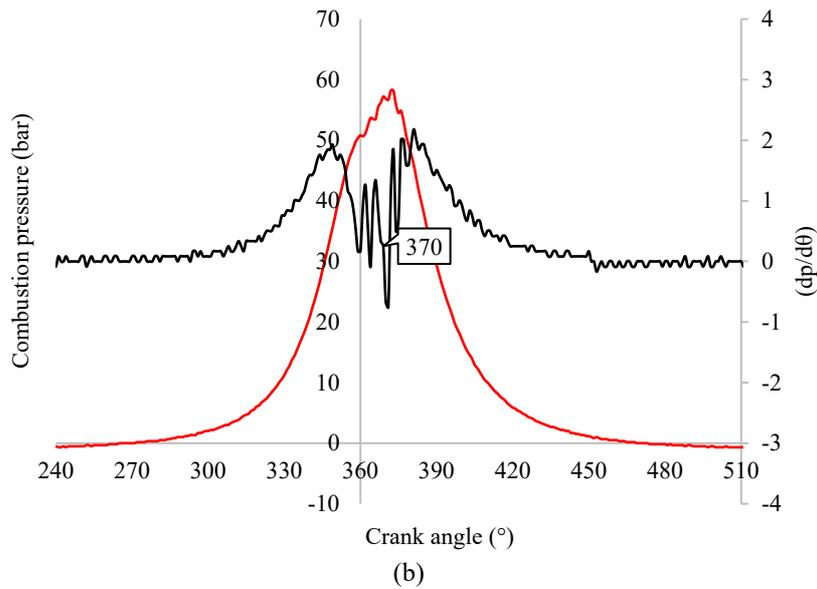
**Figure 6.** (a) Diesel and (b) PJME combustion pressure derivative at 50% engine load.
