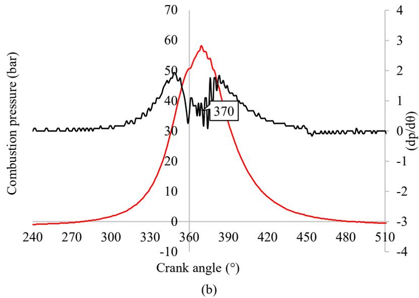
**Figure 5.** (a) Diesel and (b) PJME combustion pressure derivative at 75% engine load.
