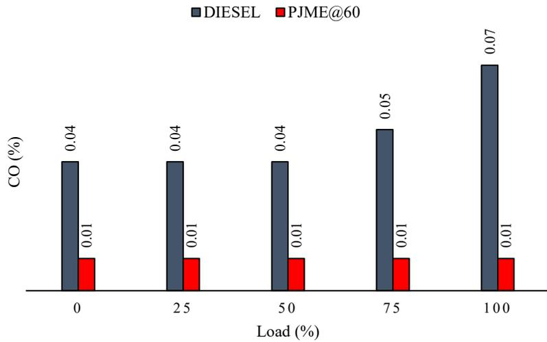
Figure 10. CO vs engine load.
