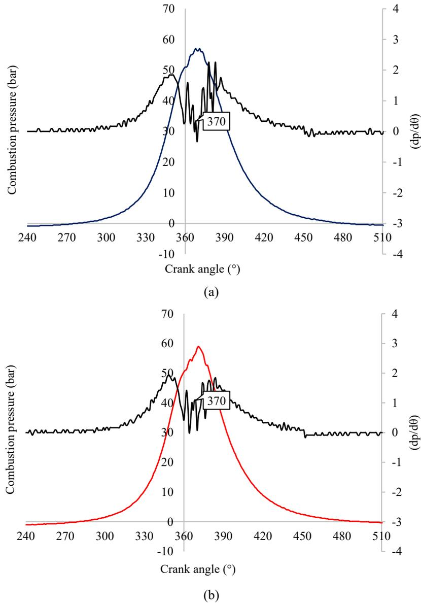
**Figure 4.** (a) Diesel and (b) PJME combustion pressure derivative at 100% engine load
