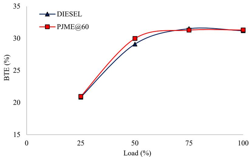
**Figure 7.** Brake thermal efficiency vs. engine load.
