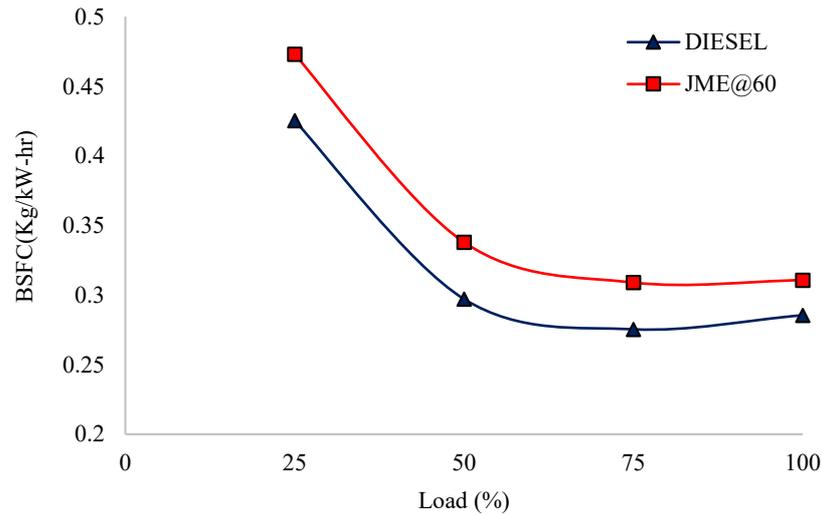
Figure 8. BSFC vs. engine load.
