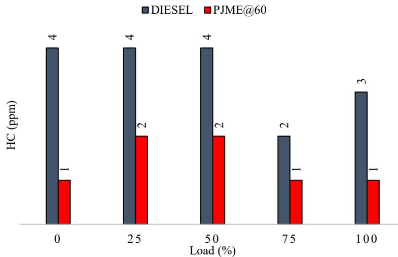
Figure 9. HC vs. engine load.
