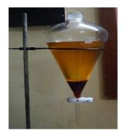
Figure 1. Jatropha biodiesel and glycerin separation.
