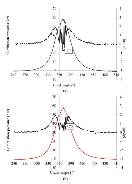
Figure 5. (a) Diesel and (b) PJME combustion pressure derivative at 75% engine load.
