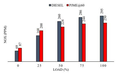
Figure 12. NO vs engine load.
