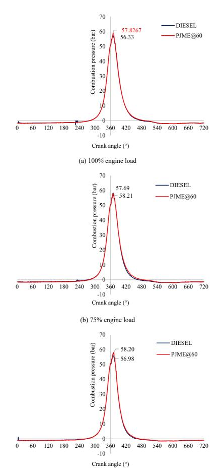
(c) 50% engine load Figure 3. Combustion pressure at different engine loads.
