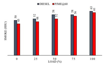
Figure 13. Smoke vs. engine load.
