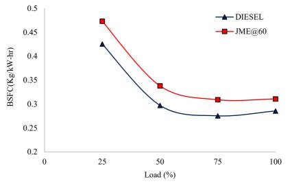
Figure 8. BSFC vs. engine load.
