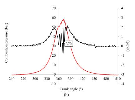
Figure 6. (a) Diesel and (b) PJME combustion pressure derivative at 50% engine load.
