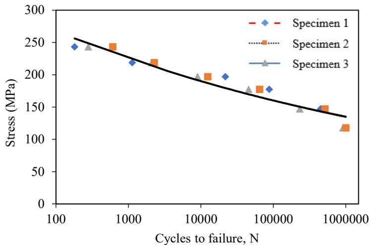
**Figure 2.** Experimental fatigue S-N curve of glass/epoxy composite under tension-tension fatigue test with R=0.1.
