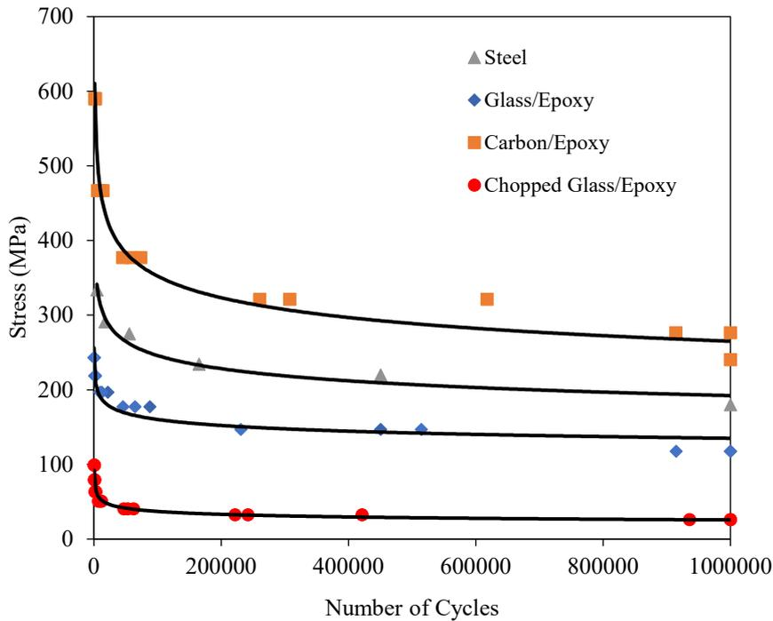
**Figure 6.** Number of cycles with applied stress comparison between steel and composite materials.
