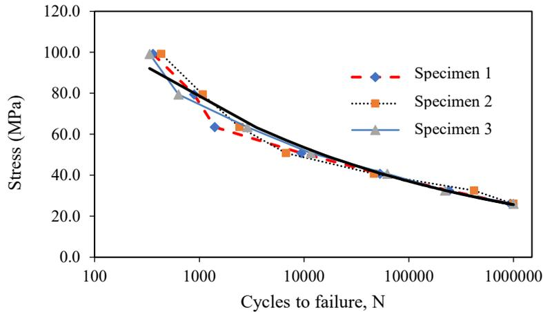
**Figure 1.** Experimental fatigue S-N curve of chopped glass/epoxy composite under tension-tension fatigue test with R=0.1.
