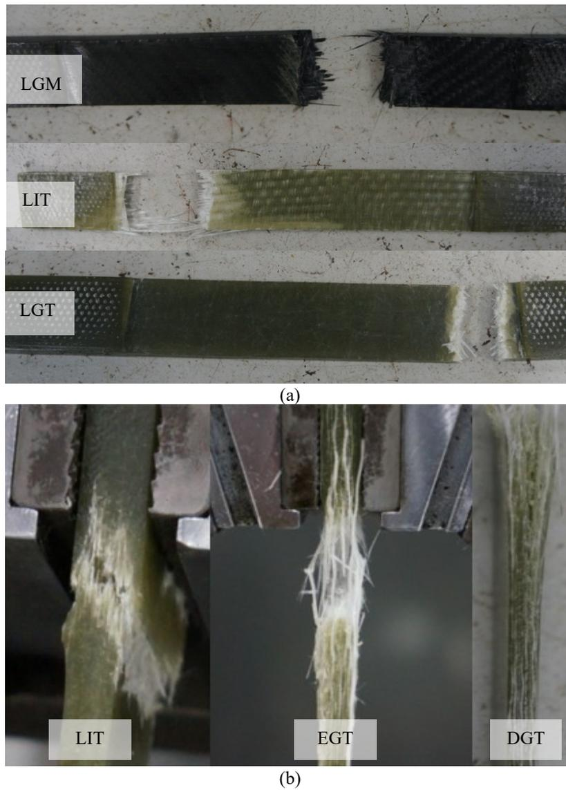
Figure 7. (a) Composite failure modes and, (b) failure mode type.
