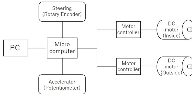
Figure 3. Inner and outer wheels driving force control system.
