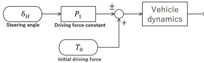
Figure 2. Block diagram of inner and outer wheels driving force control system based on the steering angle.
