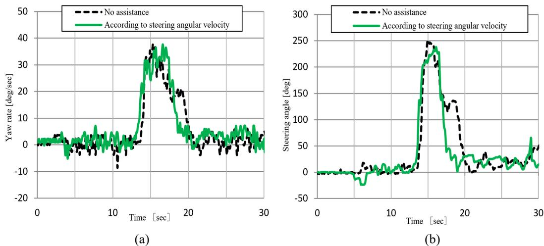
**Figure 12.** Comparison between Steering angular velocity control and no assistance during J-turn driving (a) yaw rate and (b) steering angle
