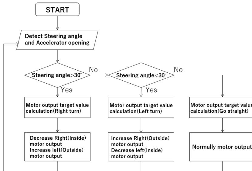
Figure 4. Flow chart of inner and outer wheels driving force control system.
