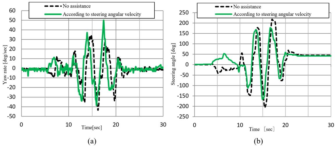
**Figure 9.** Comparison between Steering angular velocity control and no assistance during pylon slalom driving (a) yaw rate (b) steering angle.
