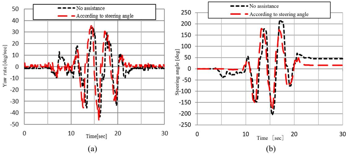
**Figure 8.** Comparison between steering angle proportional control and no assistance during pylon slalom driving (a) yaw rate and (b) steering angle.
