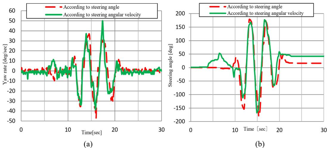
**Figure 10.** Comparison between steering angle proportional control and Steering angular velocity control during pylon slalom driving (a) yaw rate (b) steering angle.
