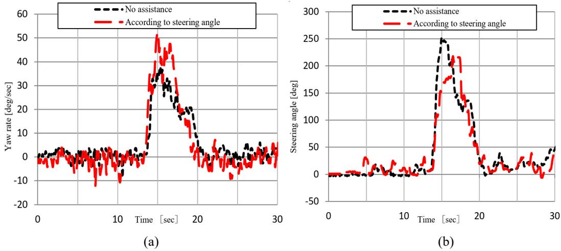
**Figure 11.** Comparison between steering angle proportional control and no assistance during J-turn driving (a) yaw rate and (b) steering angle.
