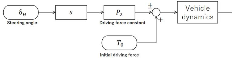
**Figure 5.** Block diagram of the inner and outer wheels driving force control system based on steering angular velocity.
