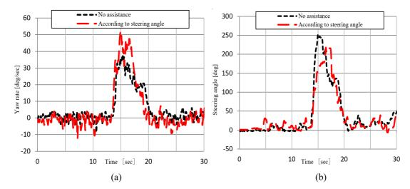
Figure 11. Comparison between steering angle proportional control and no assistance during J-turn driving (a) yaw rate and (b) steering angle.
