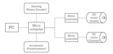
Figure 3. Inner and outer wheels driving force control system.
