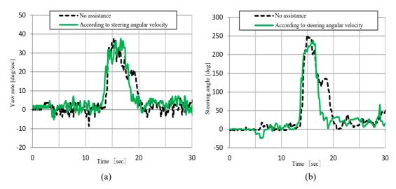
Figure 12. Comparison between Steering angular velocity control and no assistance during J-turn driving (a) yaw rate and (b) steering angle
