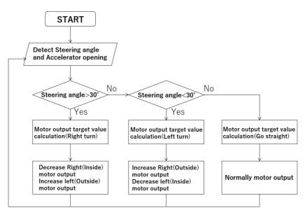
Figure 4. Flow chart of inner and outer wheels driving force control system.
