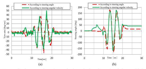
Figure 10. Comparison between steering angle proportional control and Steering angular velocity control during pylon slalom driving (a) yaw rate (b) steering angle.
