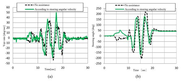
Figure 9. Comparison between Steering angular velocity control and no assistance during pylon slalom driving (a) yaw rate (b) steering angle.
