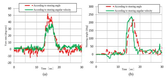
Figure 13. Comparison between steering angle proportional control and Steering angular velocity control during J-turn driving (a) yaw rate (b) steering angle
