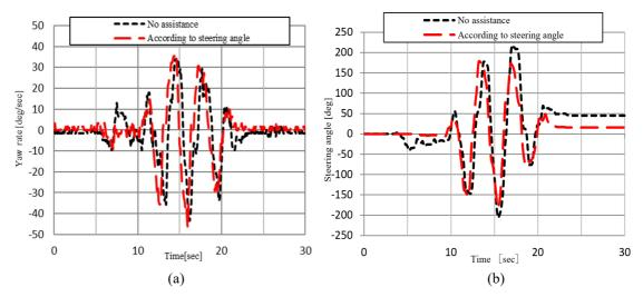
**Figure 8.** Comparison between steering angle proportional control and no assistance during pylon slalom driving (a) yaw rate and (b) steering angle.
