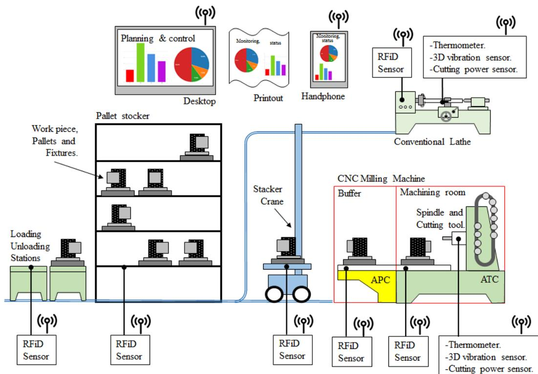
Figure 4. The sensor network in the manufacturing systems.
