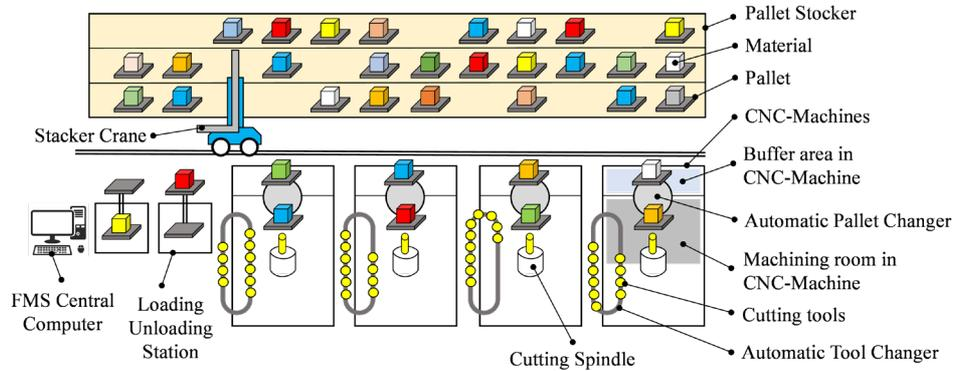
Figure 1. The FMS construction.
