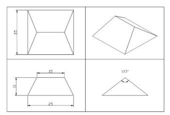
Figure 1. 3D model design of single trapezoidal folded lobe (all dimensions are in mm).
