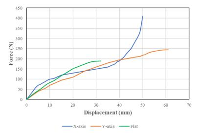
Figure 11. Force-displacement curves of compression in x-axis and y-axis direction.
