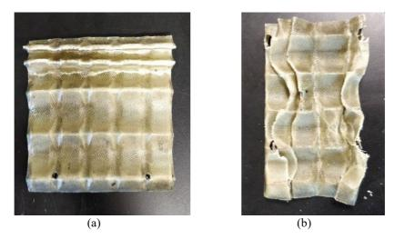
Figure 10. Sample compressed in (a) y-axis direction and (b) x-axis direction.
