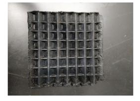
Figure 4. Trapezoidal folded lobe rubber mould (female).
