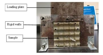
Figure 7. Setup for compression test.
