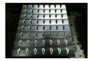
Figure 3. Trapezoidal folded lobe aluminium mould (male).
