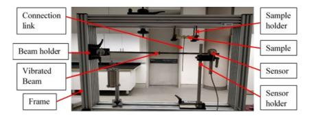
Figure 6. Setup for free vibration test.
