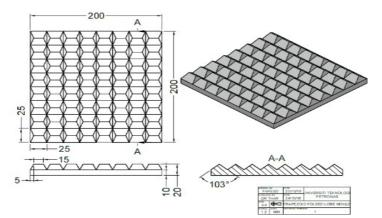
Figure 2. 3D model design of trapezoidal folded lobe shape mould (all dimensions are in mm).
