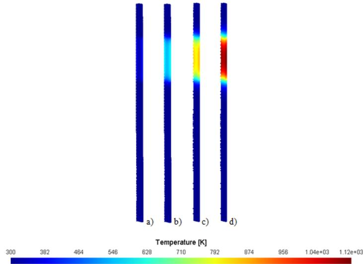
**Figure 3.** Exemplary temporary temperature distributions in the column for (a)  $t=10$  s, (b)  $t=50$  s, (c)  $t=100$  s, and (d)  $t=150$  s at system parameters of  $d=0.03$  m,  $l=1$  m,  $l_l=0.75$  m,  $q_b=200000$  W/m<sup>2</sup>,  $h=0.2$  m.
