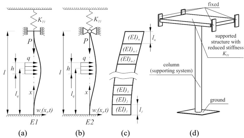
**Figure 4.** The scheme of the column subjected to the Euler’s load and local heat source: (a) column E1, (b) column E2, (c) column divided into segments and (d) representation of the real system.
