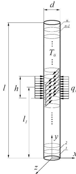
**Figure 1.** Diagram of the system of the heat-loaded column.
