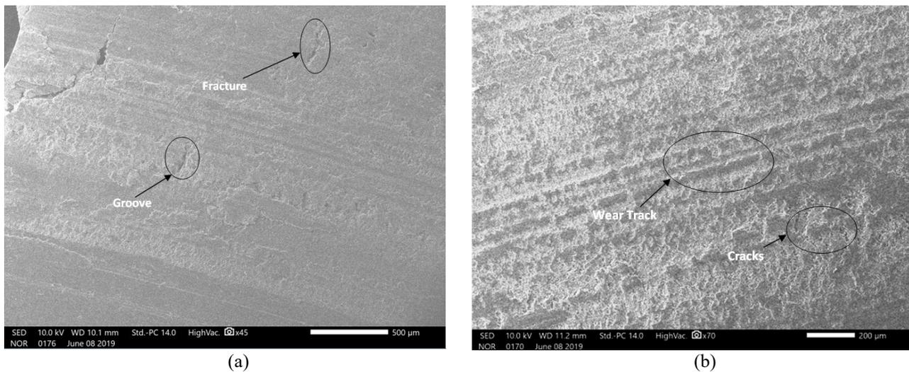
**Figure 10.** Wear tested SEM image at 200 microns of (a) 200 gsm and (b) 240 gsm fibre reinforced composites.
