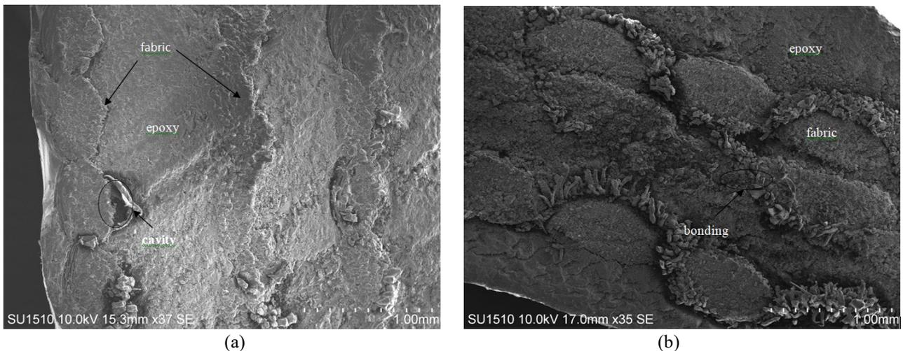
**Figure 9.** Fractured SEM image of (a) 200 gsm and (b) 240 gsm fibre reinforced composites.
