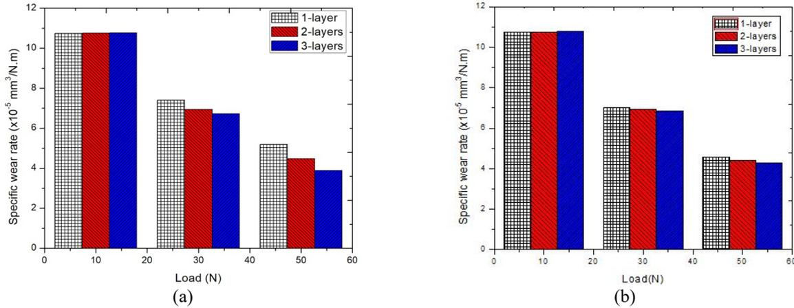
**Figure 8.** Variation of SWR at different loads for (a) 200 gsm and (b) 240 gsm of UHMWPE fibre reinforced composite specimens.
