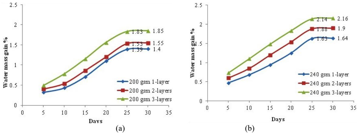
**Figure 3.** Water absorption test results for (a) 200 gsm and (b) 240 gsm specimens.
