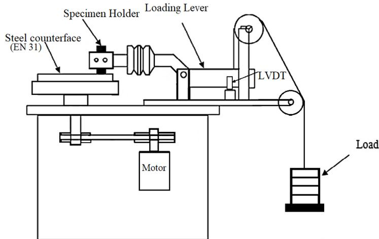
**Figure 1.** Schematic diagram of wear test rig.
