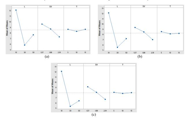
Figure 4. Main effect plot of 200 gsm at (a) 1-layer, (b) 2-layers and (c) 3-layers fabric reinforced composites for specific wear rate.
