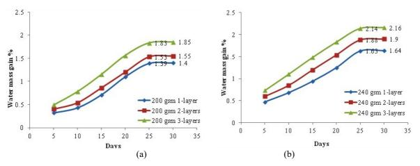
Figure 3. Water absorption test results for (a) 200 gsm and (b) 240 gsm specimens.
