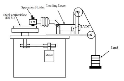
Figure 1. Schematic diagram of wear test rig.
