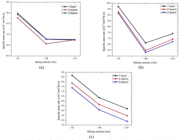
Figure 6. Variation of SWR for 200 gsm fibre reinforced composites at (a) 10 N, (b) 30 N and (c) 50 N load.
