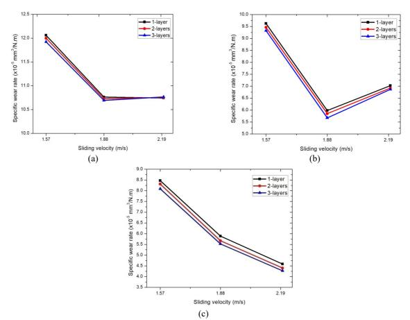
Figure 7. Variation of SWR for 240 gsm fibre reinforced composites at (a) 10 N, (b) 30 N and (c) 50 N load.
