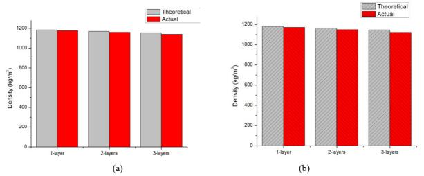
Figure 2. Theoretical and actual density of composite laminate at (a) 200 gsm and (b) 240 gsm.
