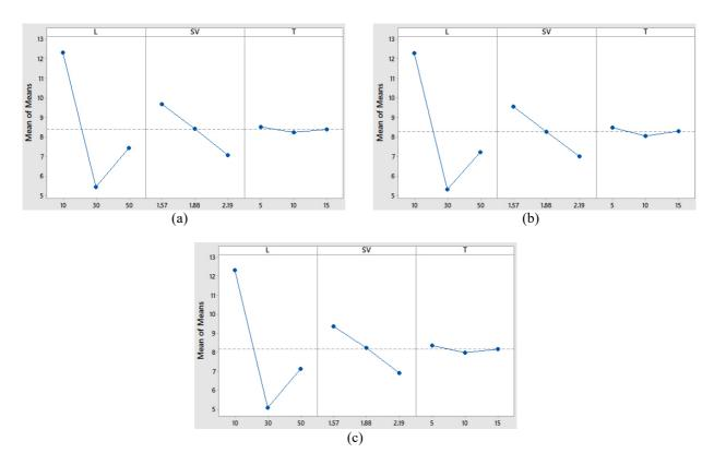
Figure 5. Main effect plot of 240 gsm at (a) 1-layer, (b) 2-layers and (c) 3-layers fabric reinforced composites for specific wear rate.
