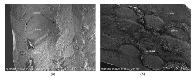
Figure 9. Fractured SEM image of (a) 200 gsm and (b) 240 gsm fibre reinforced composites.
