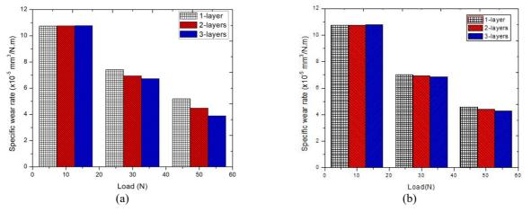
Figure 8. Variation of SWR at different loads for (a) 200 gsm and (b) 240 gsm of UHMWPE fibre reinforced composite specimens.
