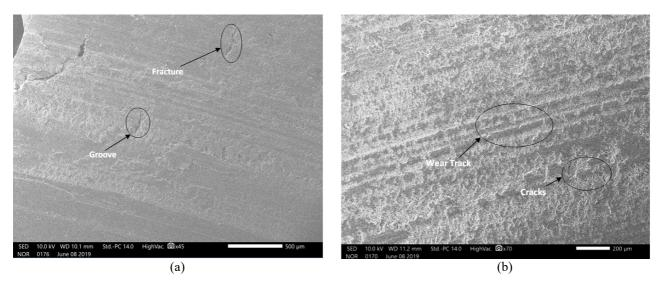
Figure 10. Wear tested SEM image at 200 microns of (a) 200 gsm and (b) 240 gsm fibre reinforced composites.
