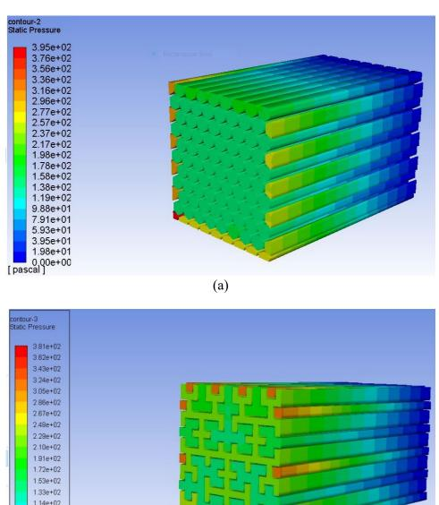
Figure 7. Pressure contour of (a) honeycomb and (b) the proposed fractal curve model.
