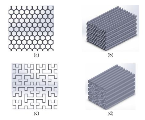
Figure 4. A 2-D and 3-D model of honeycomb (a), (b) and proposed structure (c), (d).
