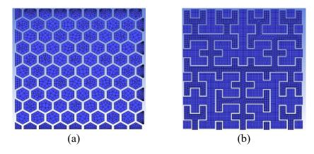
Figure 5. Meshed (a) honeycomb model and (b) proposed fractal curve model.
