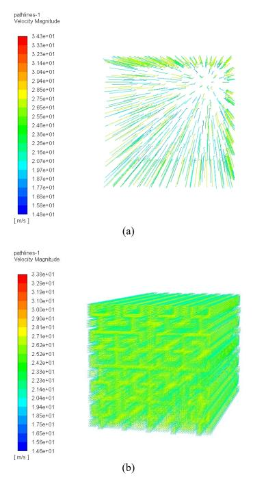
Figure 10. Flow distribution of (a) honeycomb and (b) proposed fractal curve model.
