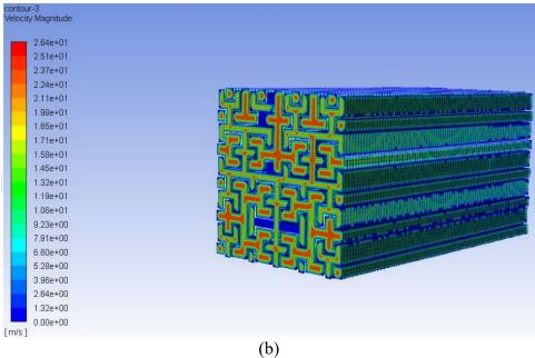
Figure 9. Velocity contour of (a) honeycomb and(b) proposed fractal curve model.
