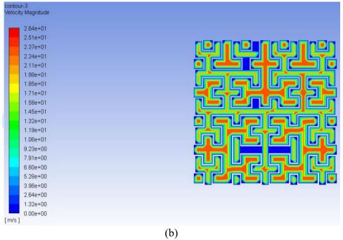
Figure 8. Velocity contour of (a) honeycomb and (b) proposed fractal curve model at inlet.
