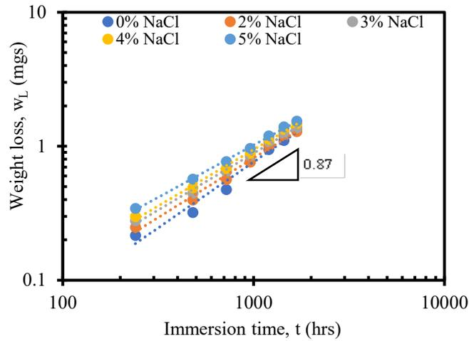
**Figure 3.** Effect of immersion times on weight loss of mild steel in various of % NaCl
