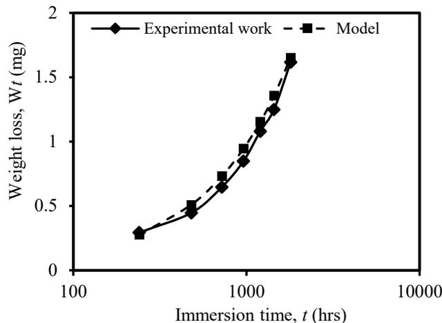
**Figure 8.** Comparison of the results of the model and the experimental work of the current study for 3 wt.% NaCl.
