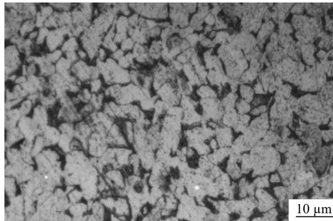
**Figure 1.** Microstructure of sample used in this study after etching using 5% nital (100 ml ethanol and 5 ml nitric acid) at ×200 magnification.
