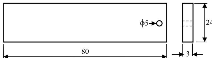
**Figure 2.** Shape and size of the sample (all dimension in mm).
