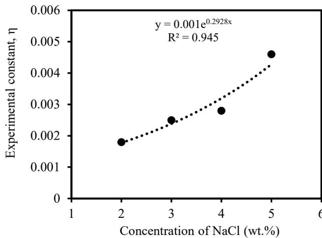
**Figure 5.** Fitting of experimental constants for various NaCl concentrations
