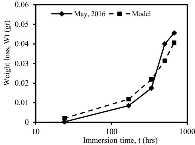
**Figure 7.** Comparison of the results of the model and experimental work of May [15] for 3 wt.% NaCl in solution.
