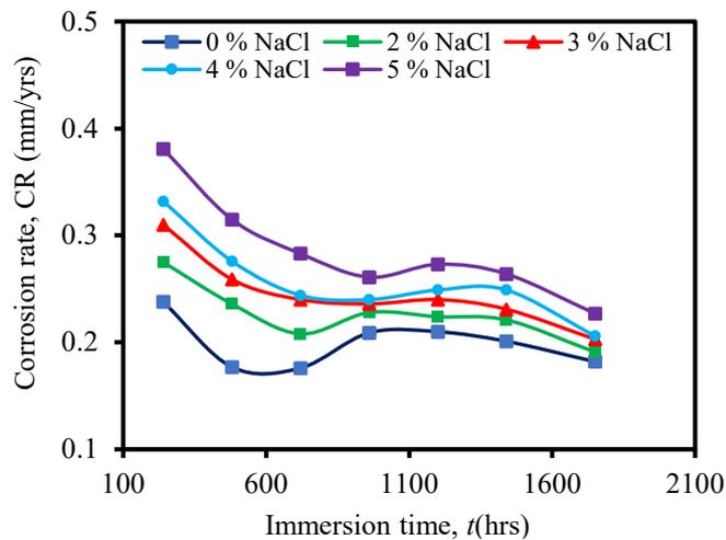
**Figure 4.** Corrosion rate versus immersion time for various NaCl concentrations.
