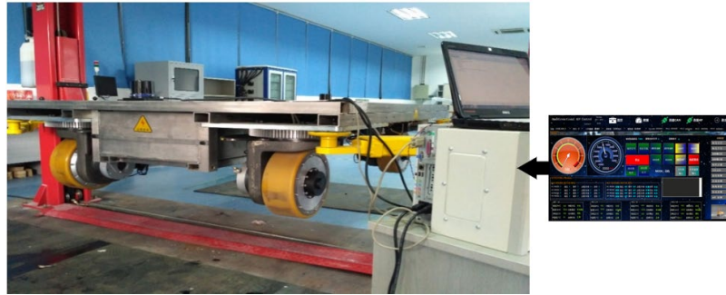
Figure 7. Experimental process of omnidirectional AGV steering angle and speed output.
