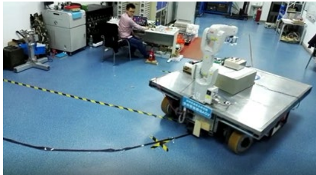
Figure 12. Circular-line tracking experiment process of omnidirectional AGV.
