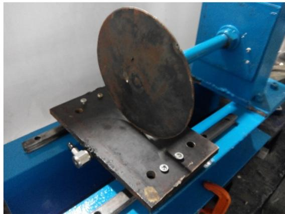
**Figure 2.** A circular plate model for experimental study.
