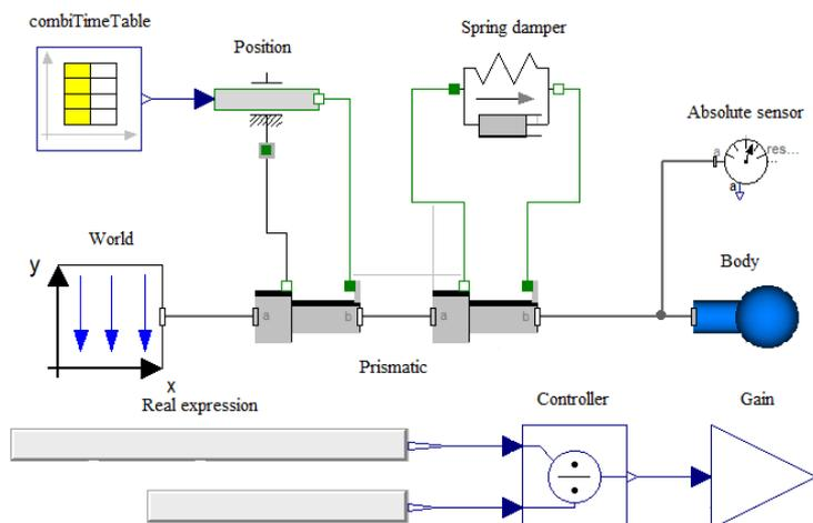
Figure 3. Diagram for strain signal simulation.
