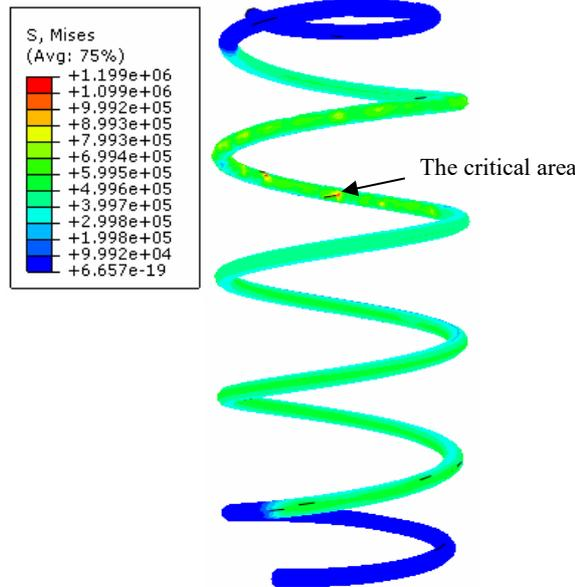
**Figure 6.** Stress distributions of the coil spring
