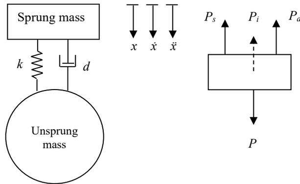
**Figure 2.** A mass-spring-damper system and its free body diagram.
