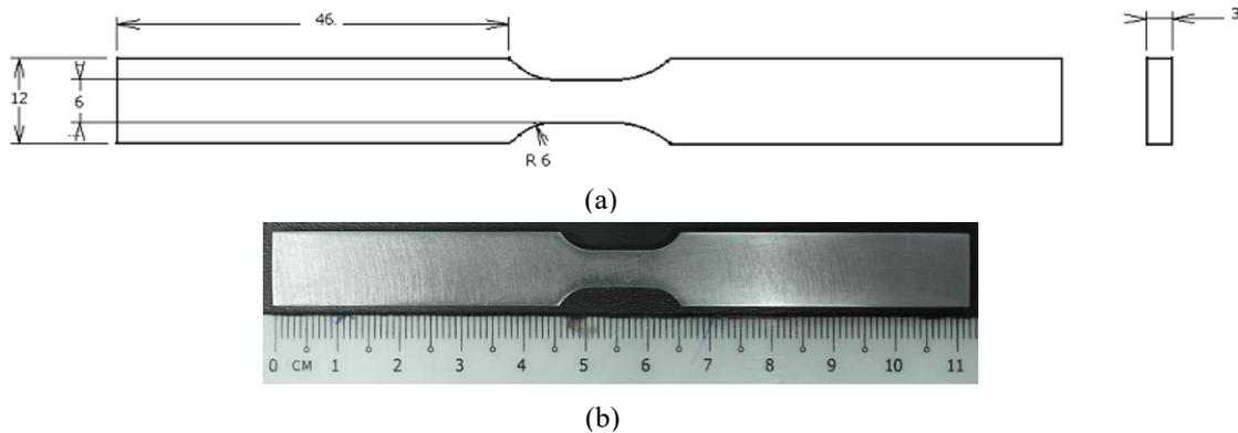
**Figure 4.** Fatigue test sample (a) geometry and dimensions in millimetres, (b) photograph.
