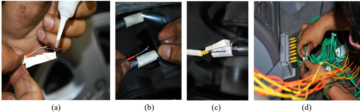
**Figure 1.** The strain gauge installation: (a) applying the adhesive, (b) placing the strain gauge, (c) installing the strain gauge, and (d) connecting the sensor to the data acquisition.
