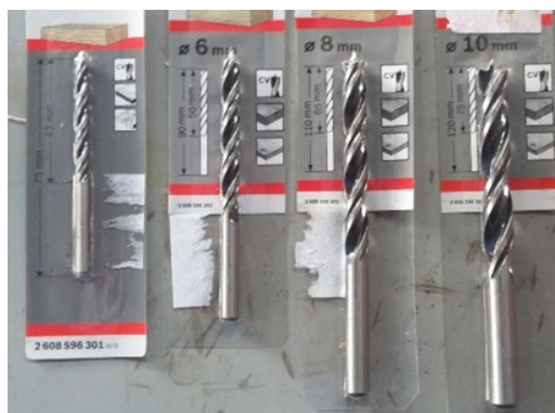
Figure 2. "Brad & spur" drill diameter 4, 6, 8 and 10 mm.
