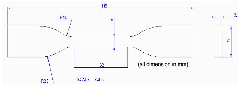
Figure 2. Specimen design according to ASTM D638.
