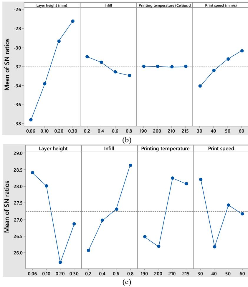
Figure 4. Mean S/N ratio versus parameters for (a) weight, (b)printing time and (c) tensile strength.
