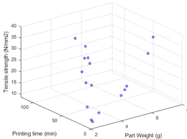
**Figure 9.** Pareto front of weight, printing time and tensile strength optimisation.
