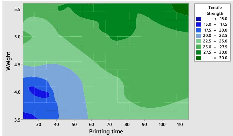
Figure 7. Contour plot of tensile strength vs. weight vs. printing time.
