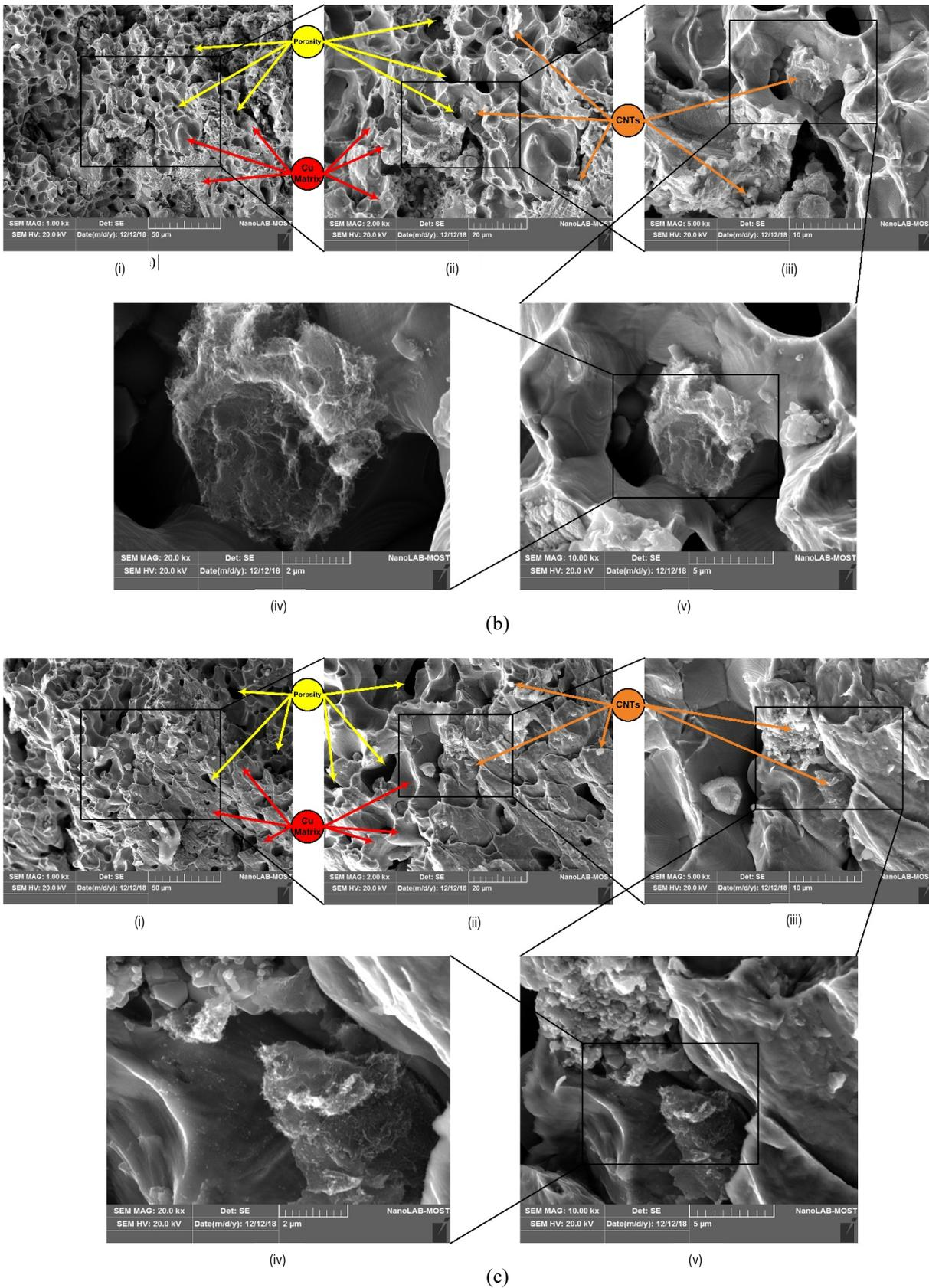
Figure 2. SEM views of (a) Cu/Fe - 0% CNTs, (b) Cu/Fe - 0.6 % CNTs, (c) Cu/Fe - 1.2 % CNTs.
