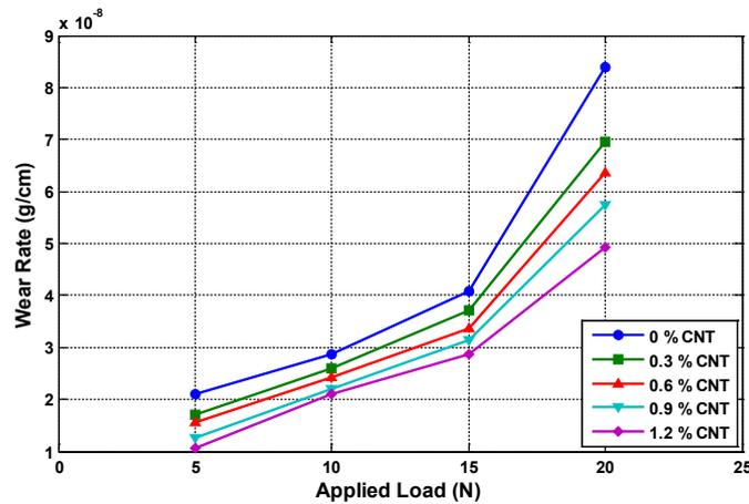
Figure 6. Variation of wear rates of the hybrid composites with varying applied loads.
