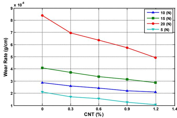
Figure 5. Variation of wear rates of the hybrid composites with the different volume fraction of CNTs.
