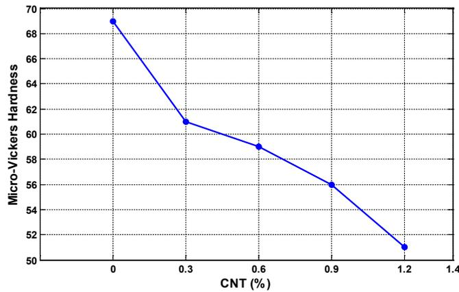
Figure 4. Variation of microhardness with CNT content.
