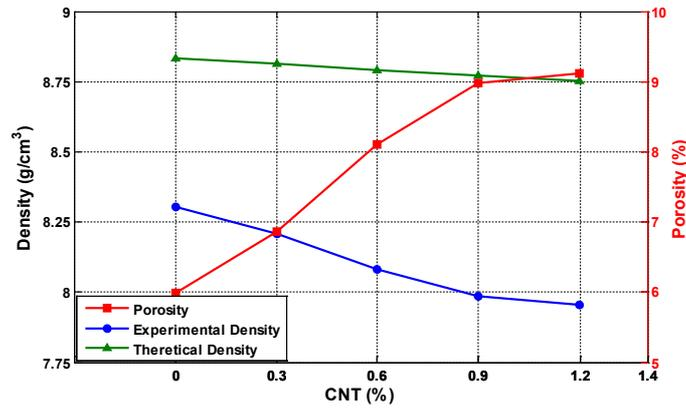
Figure 3. Variation of measured density and porosity with CNT content.
