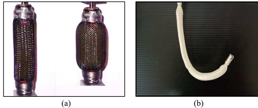
Figure 1: McKibben Actuator when under pressurised state. (a) Conventional McKibben and (b) thin McKibben.
