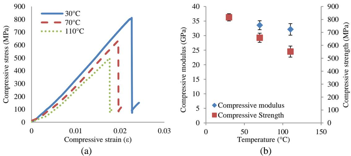
Figure 7. (a) Representative stress vs. strain curve comparison at different temperatures and (b) compressive modulus and compressive strength (with standard deviation) vs. temperature for C-0 specimens.
