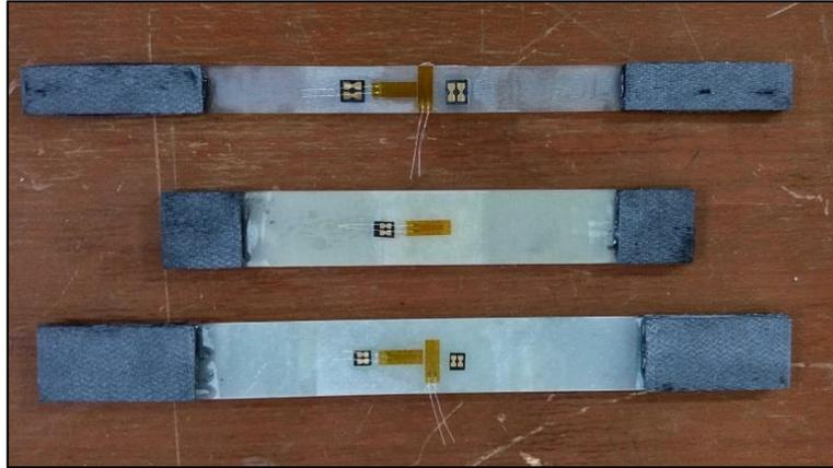
Figure 1. Specimens with tabs (in black) and strain gauges installed (from top to bottom: tensile 0°, tensile 90° and shear).
