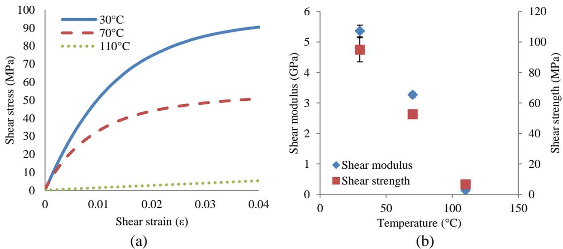
Figure 11. (a) Representative stress vs. strain curve comparison at different temperature and (b) compressive modulus and compressive strength (with standard deviation) vs. temperature for S specimens.
