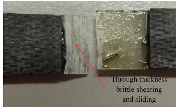
Figure 10. Failure mode of C-90 specimen.
