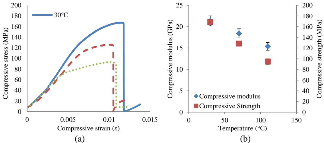
Figure 9. (a) Representative stress vs. strain curve comparison at different temperatures and (b) compressive modulus and compressive strength (with standard deviation) vs. temperature for C-90 specimens.
