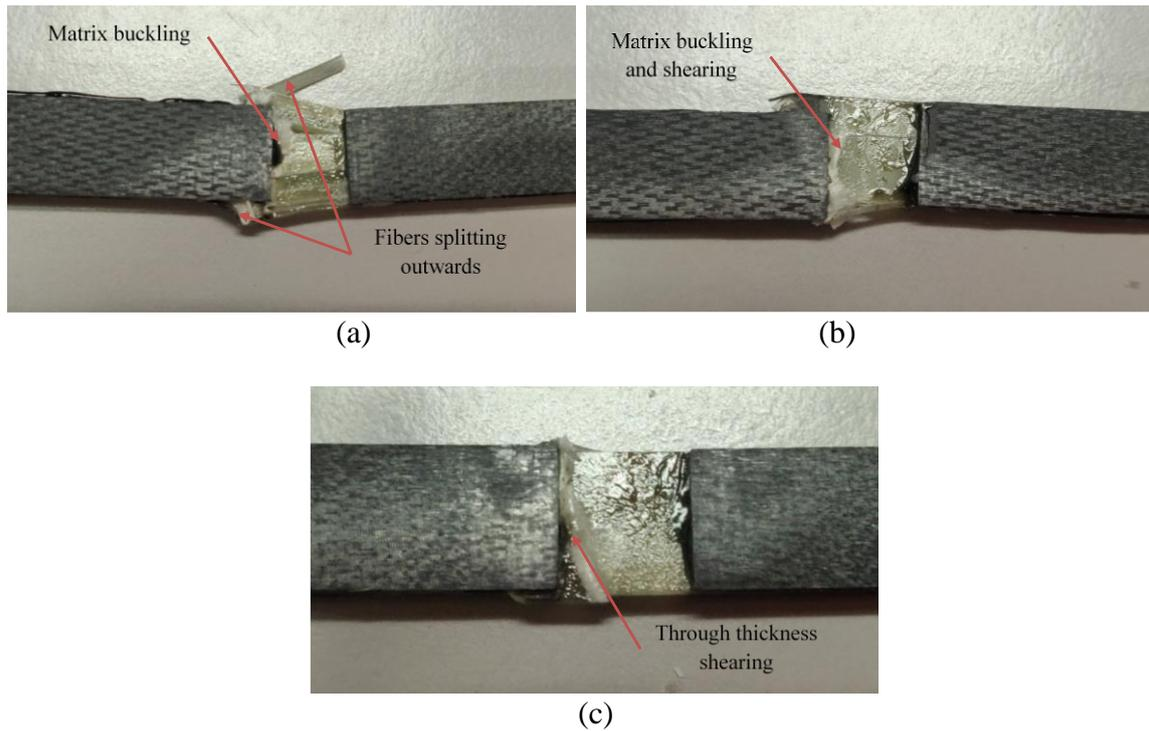
Figure 8. Failure mode of C-0 specimens tested at (a) 30°C, (b) 70°C and (c) 110°C.
