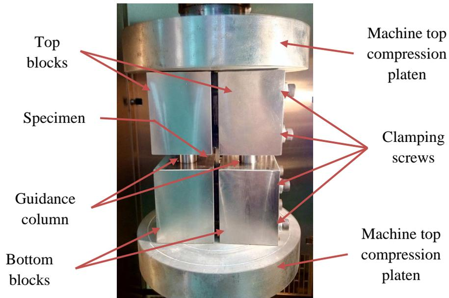
Figure 2. Compression jig setup with the specimen in between.
