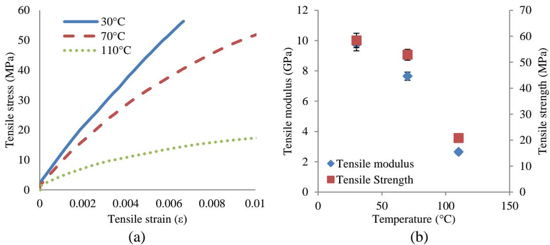
Figure 5. (a) Representative stress vs. strain curve comparison at different temperatures and (b) tensile modulus and tensile strength (with standard deviation) vs. temperature for T-90 specimens.
