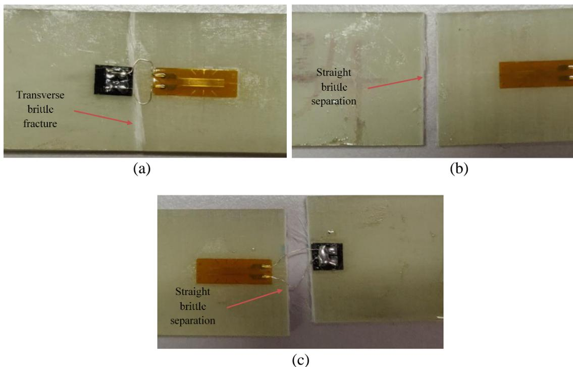
Figure 6. Failure mode of T-90 specimens tested at (a) 30°C, (b) 70°C and (c) 110°C.
