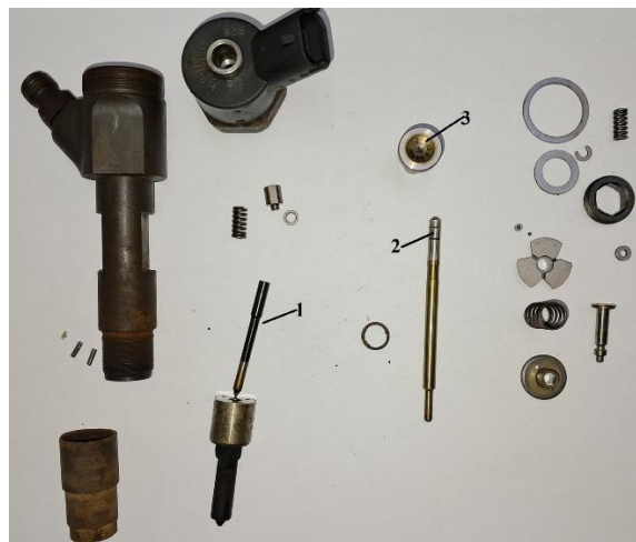
Figure 1. Components of the tested Bosch electromagnetic injector on which microscopic analysis was performed (1 - nozzle needle, 2 - control piston, 3 - valve)
