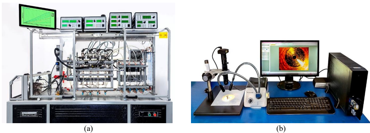
Figure 3. Measuring equipment used: a) STPiW-3 fuel injection pump and injector test bench, b) stereo microscope
