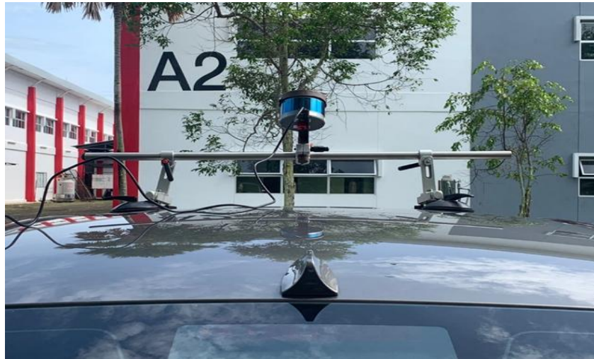
Figure 3. Installation of LiDAR sensor with metal frame on the top of the test car
