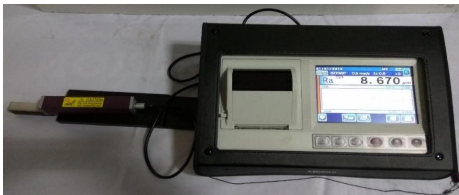
Figure 4 (a). Surface roughness measurement device Mitutoyo SJ-310
