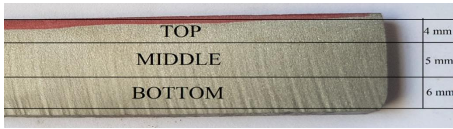
Figure 4 (b). Sample highlighting the main region for R_a value measurement
