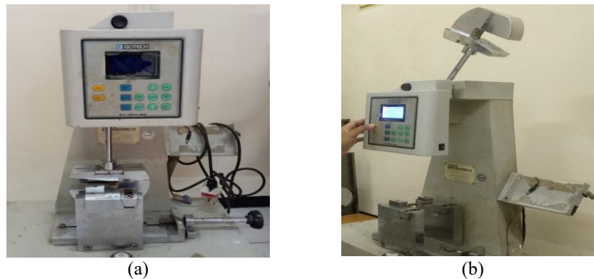
Figure 7. (a) Impact testing machine; (b) Impact testing process
