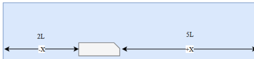
Figure 5. Enclosure of Ahmed Body in X-axis
