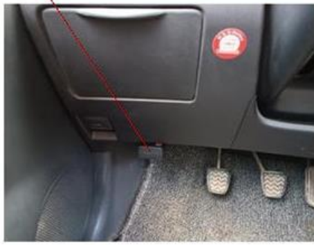
Figure 4. Connecting the Openport 2.0 Bluetooth adapter to the vehicle's DLC connector
