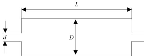
Figure 1. Muffler simple design
