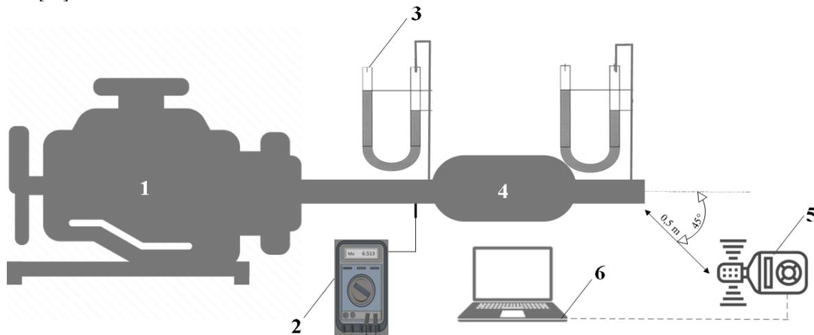
Figure 6. Schematic of test bench
