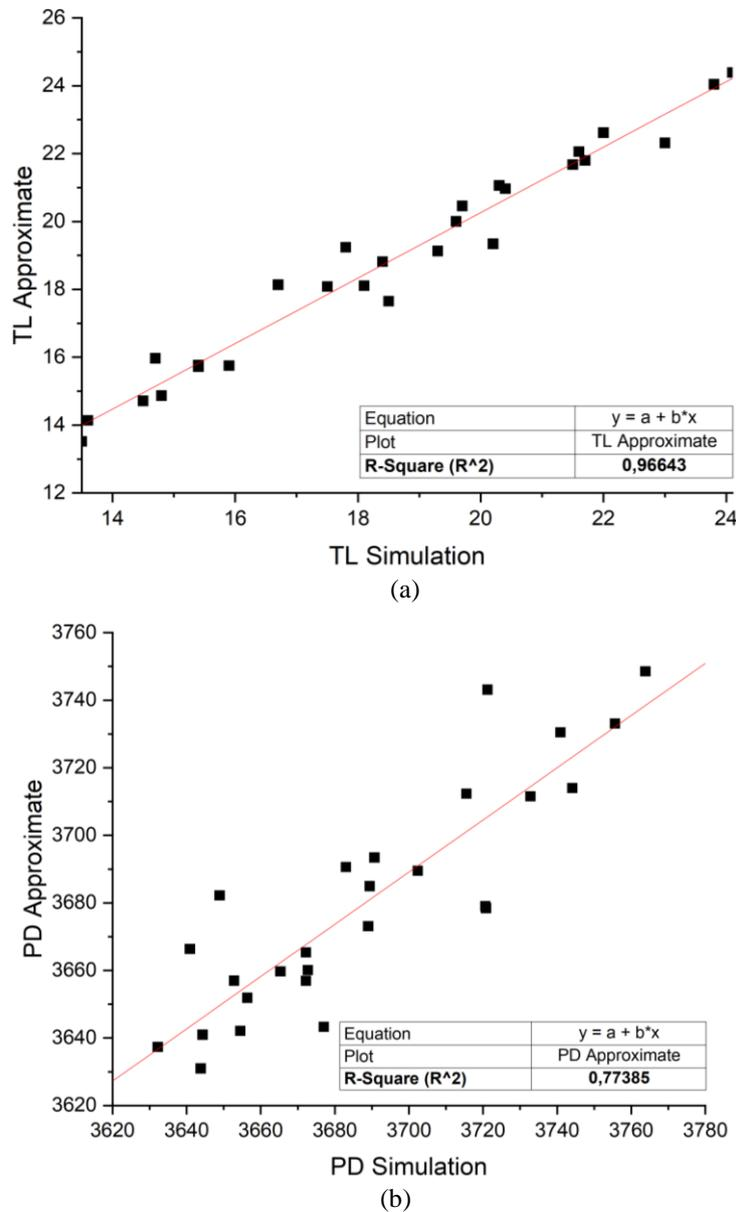
Figure 7. Determination coefficient ( $R^2$ ) of approximate model TL (a) and PD (b)
