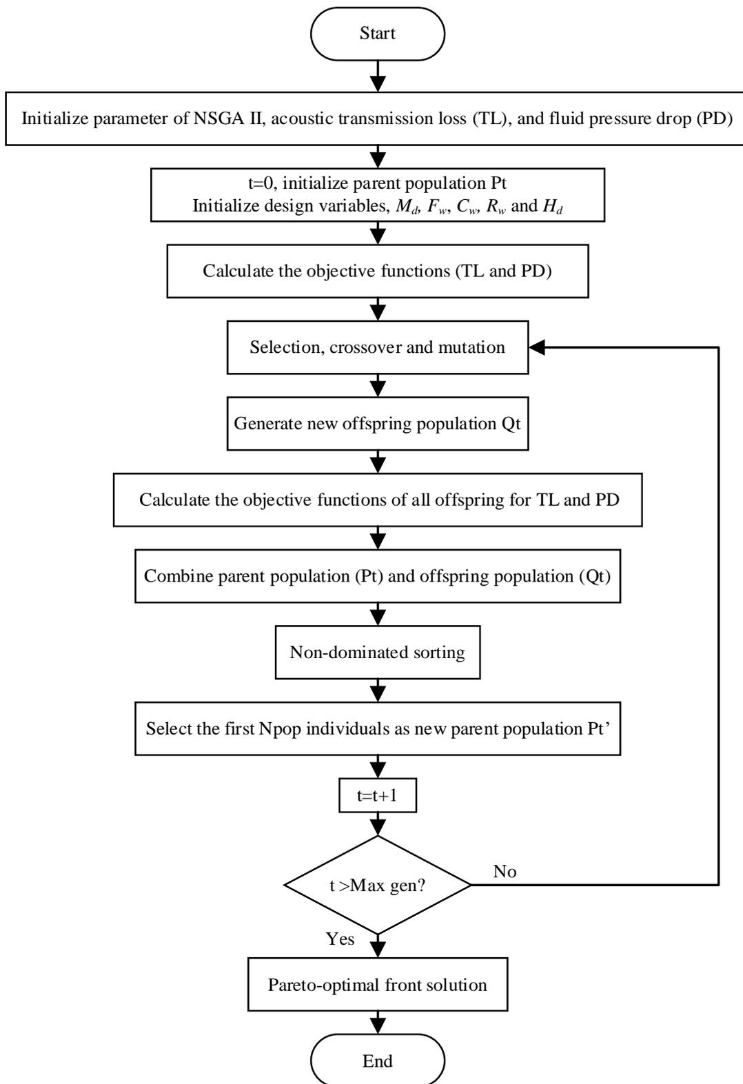
Figure 4. Flowchart of the NSGA-II algorithm
