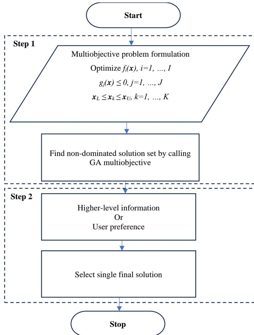
Figure 2. Two steps multiobjective optimization
