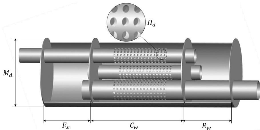
Figure 3. Design parameters for 3D three-pass perforated tube muffler visualization
