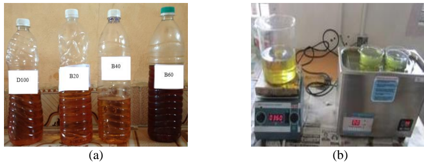
Figure 1. (a) Sample of diesel and biodiesel blends, and (b) process of adding nanoparticles in diesel and biodiesel blends
