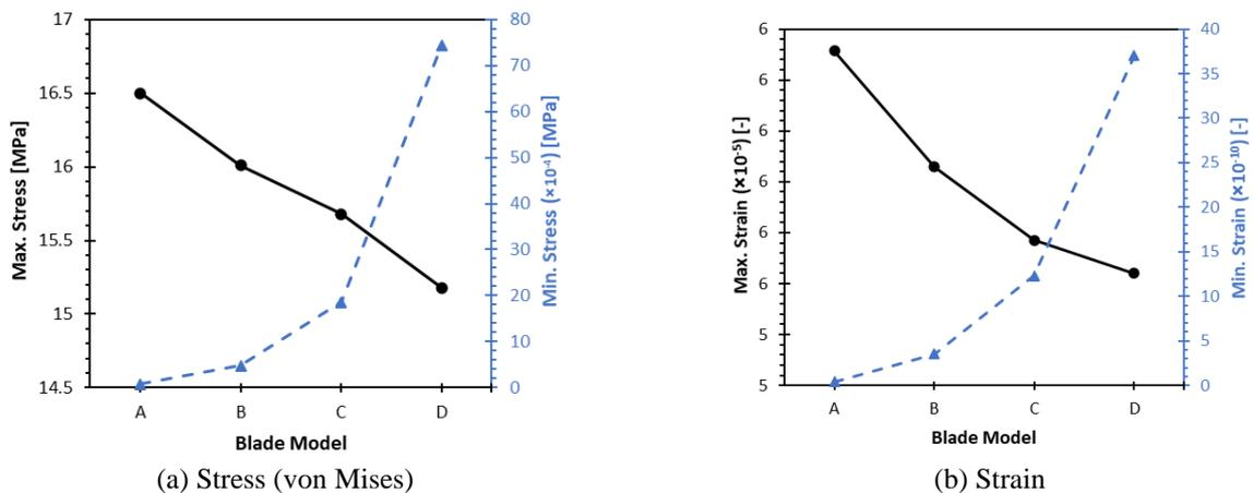
Figure 8. The maximum and minimum stress and strain of each blade model
