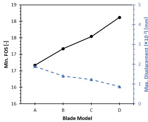
Figure 9. The minimum FOS and maximum displacement of each blade model
