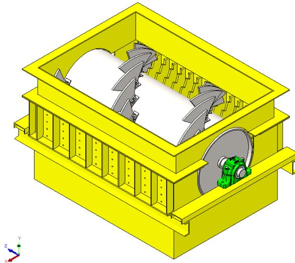
Figure 1. Drum design with blade arrangements assembled with the cutting chamber
