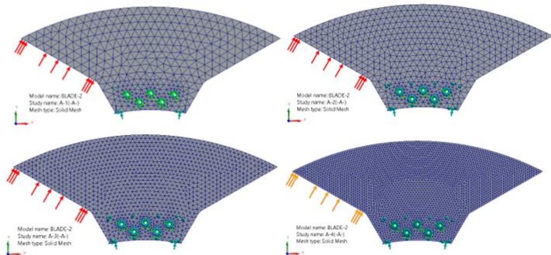
Figure 3. The generated meshes for mesh sensitivity study for blade model A
