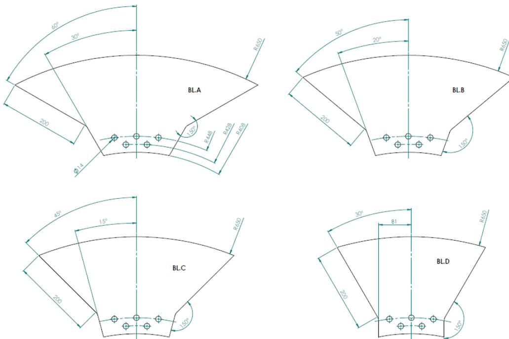
Figure 2. Different types of blade models
