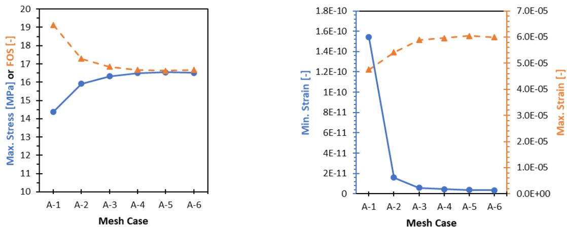
Figure 6. The effect of mesh refinement and control on the maximum stress and FOS (left) and the minimum and maximum strain (right)
