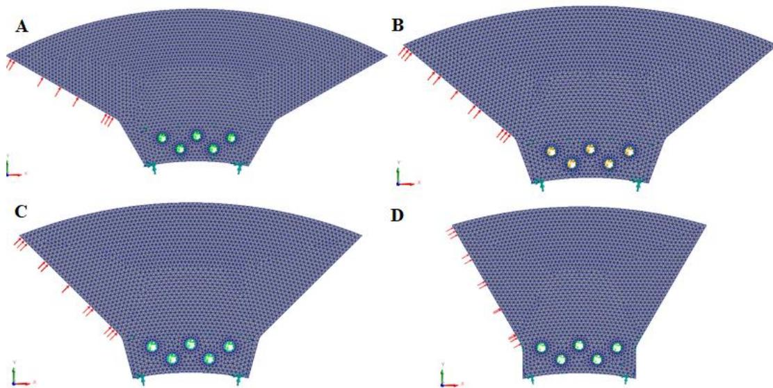
Figure 4. Mesh and Boundary conditions applied to each blade model
