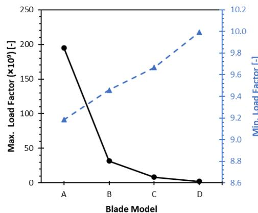
Figure 10. The minimum and maximum load factor of each blade model
